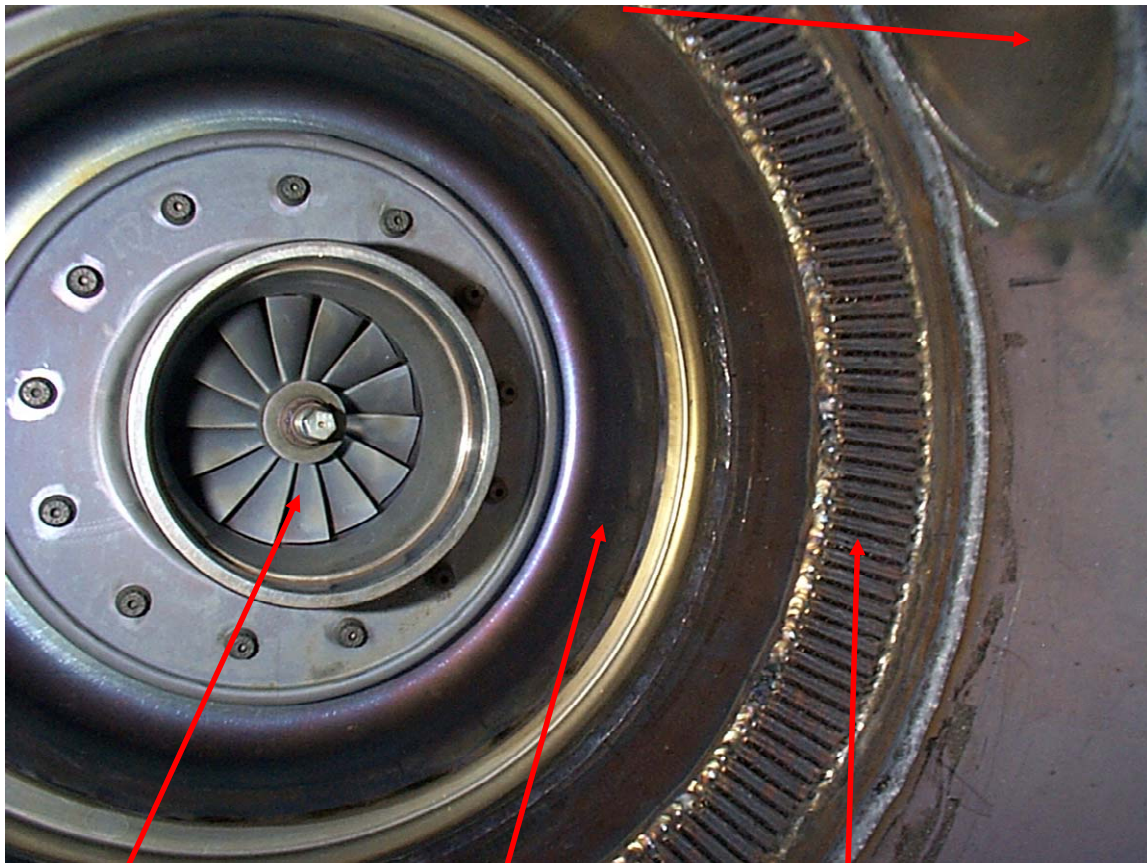
Figure 3-6: Photo of the 14 turbine exit blades, the turbine inlet annulus, and the high pressure recuperator exit. An annular shaped “combustor can” is slipped into the turbine inlet annulus to direct the gas exiting the recuperator through the injector ports to the heater.
