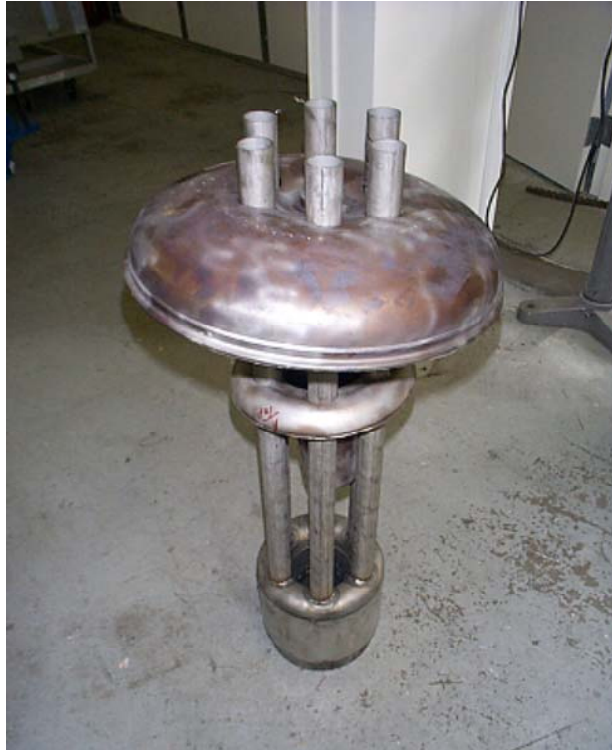
Figure 3-9: Six tubes penetrating through the turbine exit dome, through the combustor dome shaped annulus (middle “dome”), and through the turbine inlet dome (smaller bottom dome shaped annulus) .
