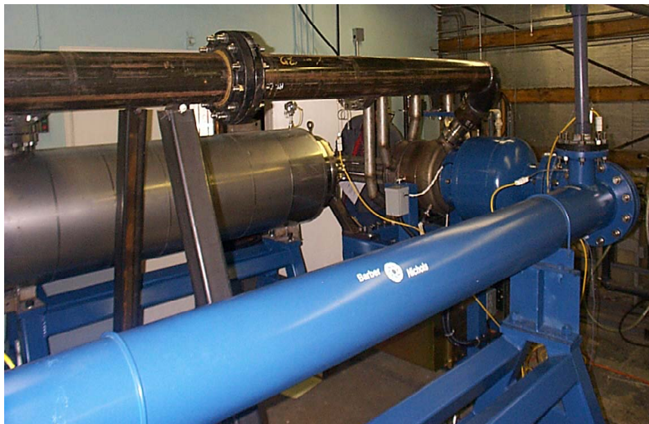
Figure 3-13: . Fully modified and assembled Capstone C-30 closed-Brayton loop as assembled at the manufactures (Barber-Nichols Inc.) is illustrated. The gas chiller is in the fore ground and the heater is on the left side of the image.
