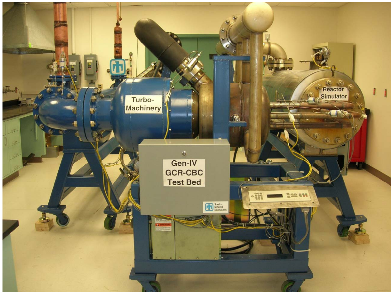
Figure 1-4: Photo of the Sandia Brayton Loop (SBL-30) installed at Sandia.
