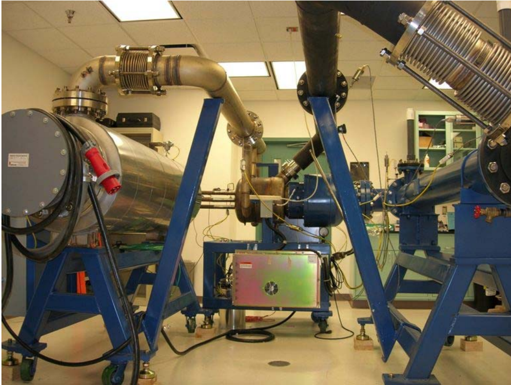
Figure 3-14: Sandia Brayton Loop as installed at Sandia. The loop is un-insulated in this figure. The heater is on the left, the gas chiller on the right, and the TAC in the middle.
