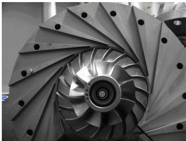
Figure 2-15: Compressor wheel and exit diffuser (left) and turbine inlet nozzle (right).
