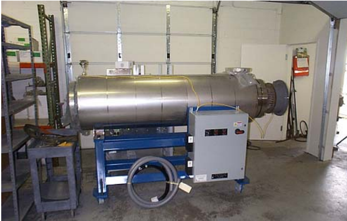
Figure 3-17: Watlow 80 kW Brayton loop gas heater and controller.
