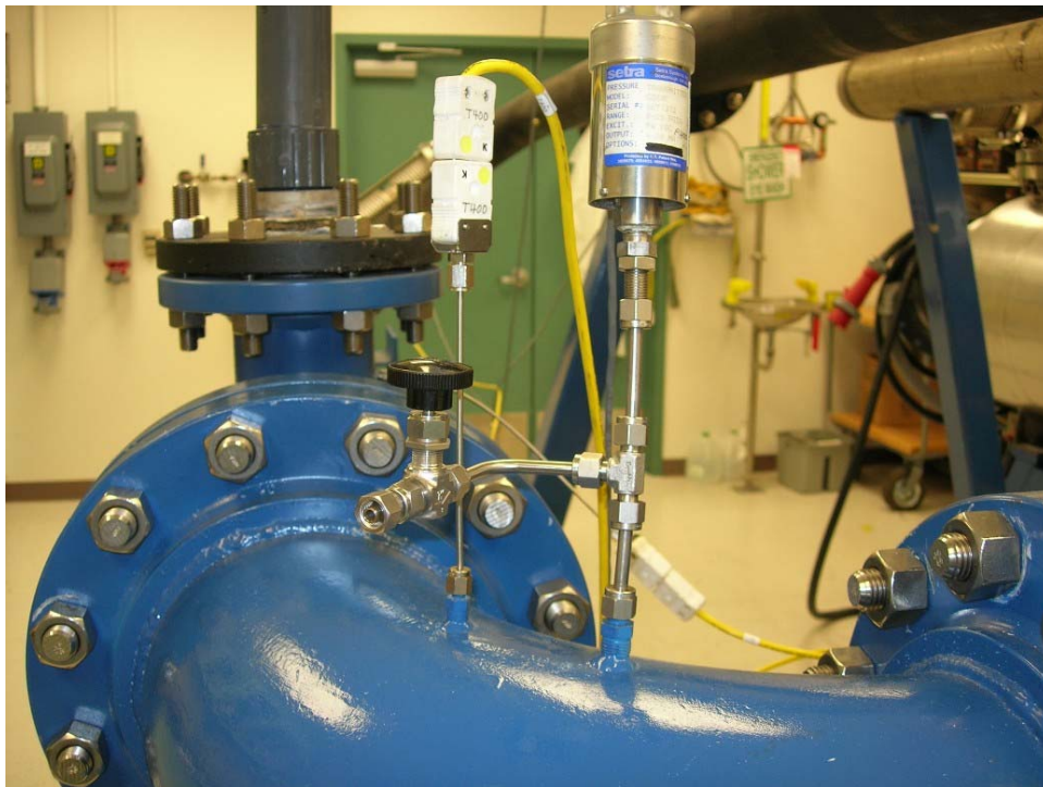
Figure 3-28 Compressor inlet temperature and pressure feed through port and sensors.
