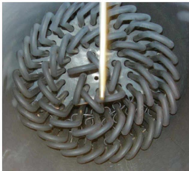
Figure 3-18: “U” shaped heater elements used in the Watlow heater. The photo shows the heater elements, the grid spacer wires, the baffle, and the gas exit thermocouple (vertical rod).
