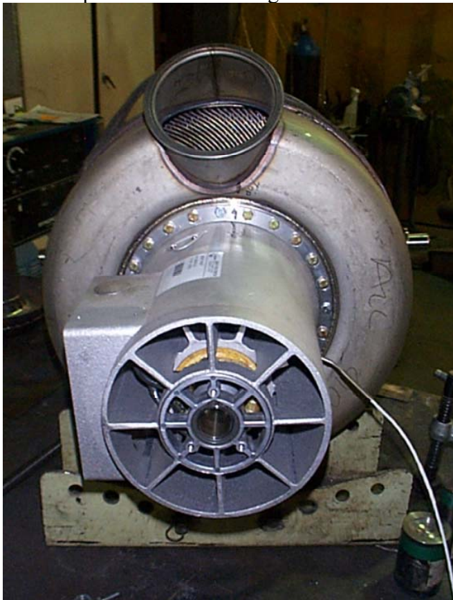
Figure 3-11: "Cold End" of the Capstone C-30 micro-turbine illustrating the spiral recuperator, the alternator, and the inlet cooling passages along the alternator.
