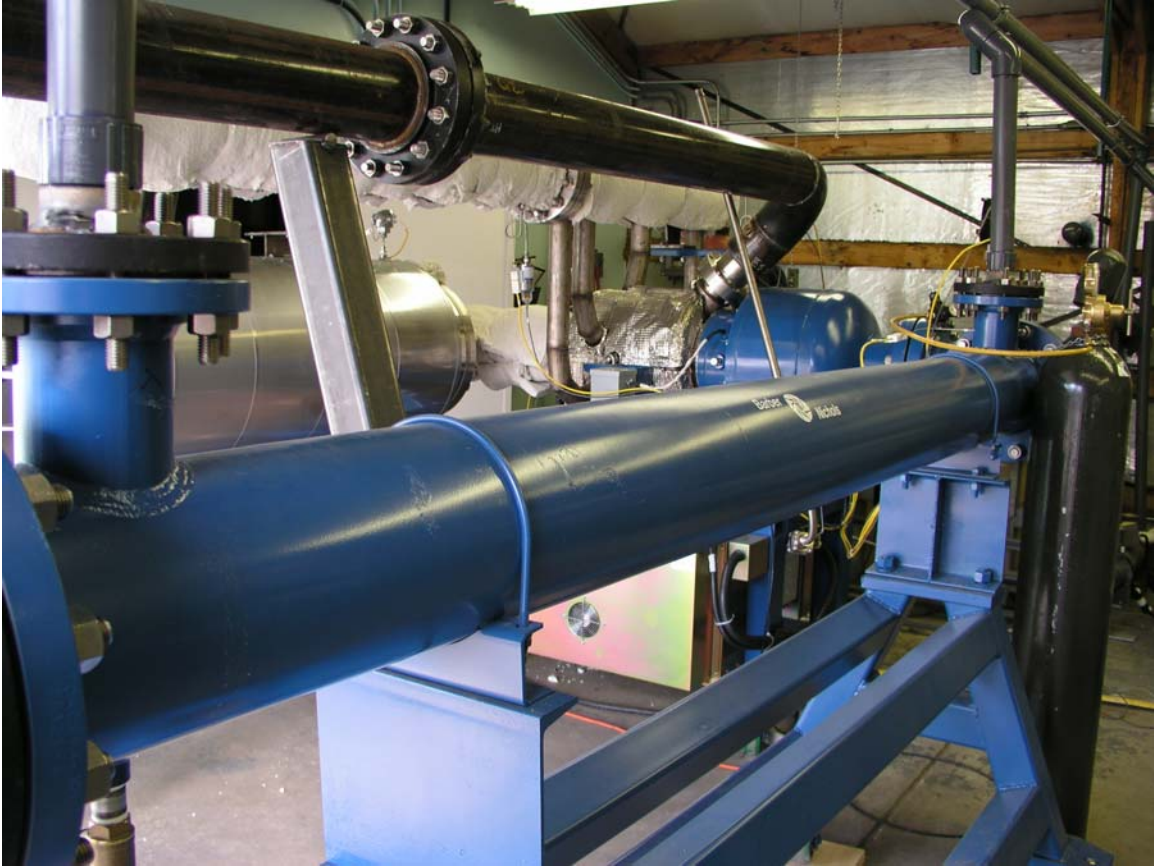
Figure 3-22: Image of the Basco/Whitlock shell and tube gas chiller. Inlet water flows from the upper right side of the image to the lower left, while gas flows in the opposite direction.
