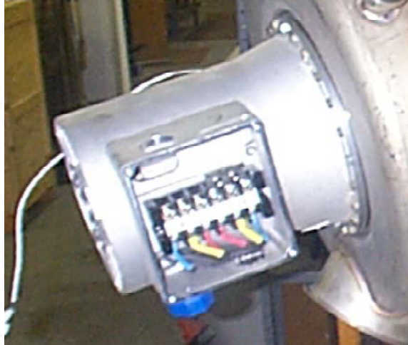
Figure 3-41: Alternator exposed electrical connections. The closest approach of two phase to phase wires is 1.6 cm.
