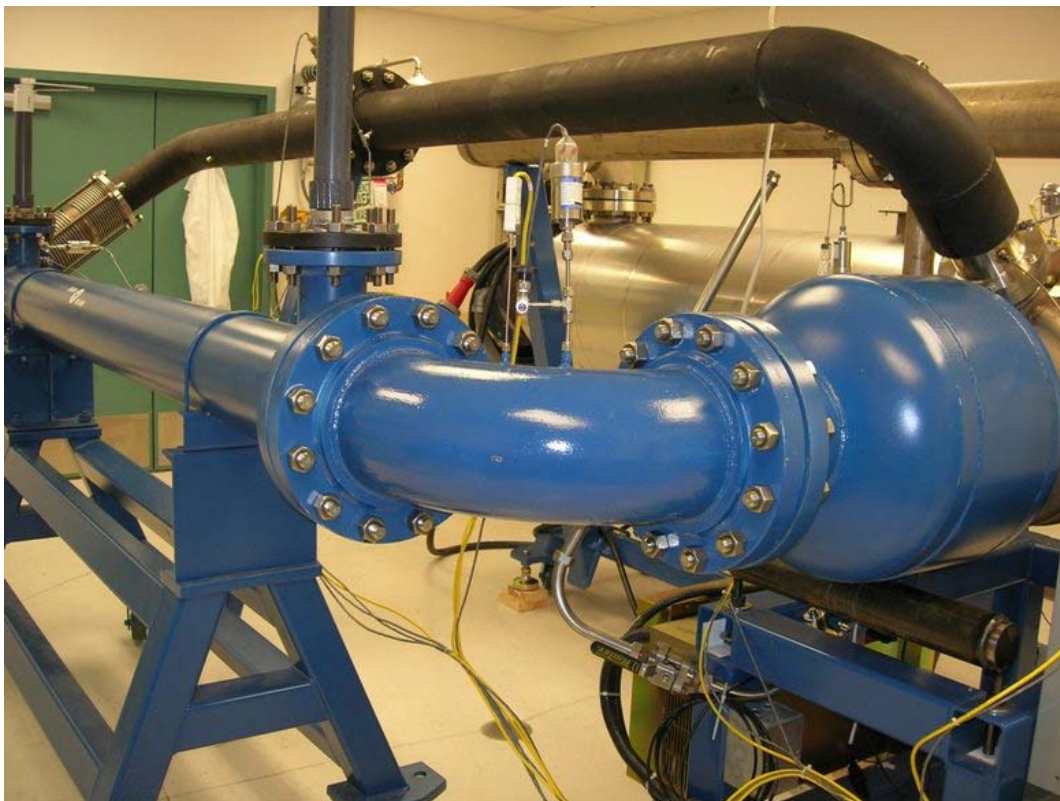
Figure 3-14: Sandia Brayton Loop as installed at Sandia. The loop is un-insulated in this figure. The heater is on the left, the gas chiller on the right, and the TAC in the middle.
