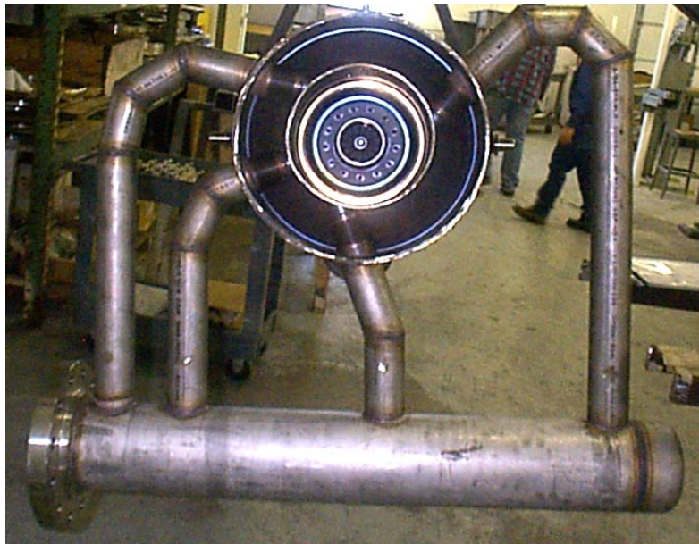
Figure 3-7: “Hot” end of the connection flow paths between the injector ports and the heat inlet duct manifold for the C-30 Capstone Micro-Turbine assembly.
