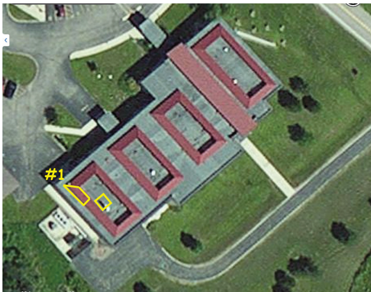
Figure 40. This aerial photograph shows the plan view of the roof. The yellow-outlined southwest-facing roof area is available for the solar thermal system discussed in this report. The outlined square near the roof area is the location of the pipe chase that goes down to the ground-level mechanical room/electrical room area. Much of the remaining roof space is preferable for a PV system.
