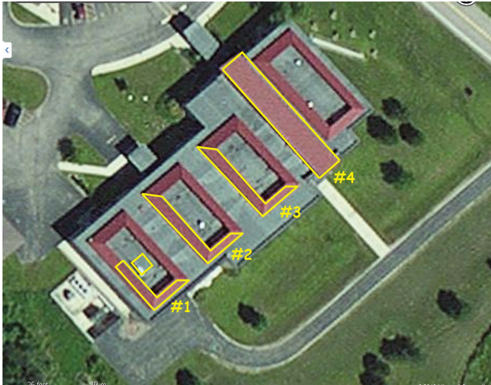
Figure 32. This aerial photograph shows the plan view of the roof. The yellow-outlined southeast- and southwest-facing roof areas are available for the PV system discussed in this report. The square in the southwest roof area is the location of the pipe chase that goes down to the ground-level mechanical room/electrical room area. The roof area not outlined in yellow on the northeast end of the building receives some shade by the atrium roof (roof area #4), and is not recommended for a solar energy system.
