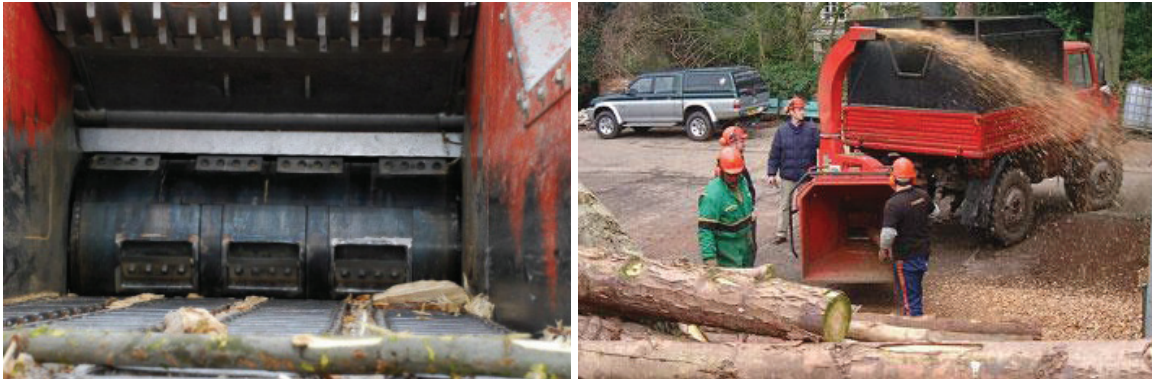
Figure 76. Potential wood chip production options. Horizontal chipper (left) and portable chipper (right).
