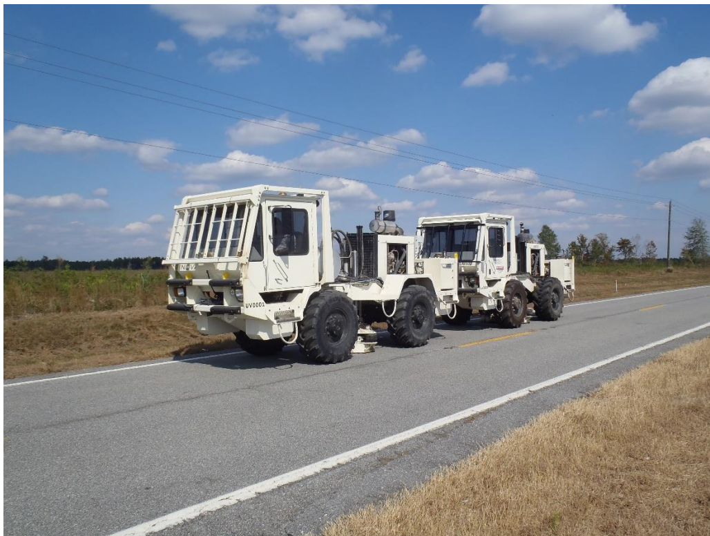
Figure 17. Two INOVA UNIVIB was used to acquire the Georgia data. These two 26,000 lbs peak force vibrators produced the same energy and frequency bandwidth as the three 42,000 lbs peak force vibrators that were used to acquire the SC data with less impact on the roads.
