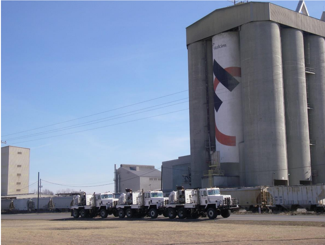
Figure 14. This figure is showing the three 42,000 lbs peak force Litton Vibrators on seismic line SCO2-4.
