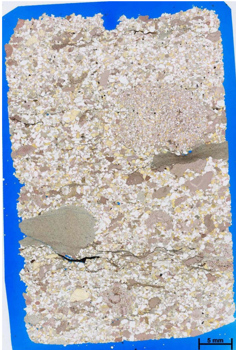
Figure 2.3 Macro photograph shows textural layering and inclined cross bedding. Potassium feldspar is stained yellow and calcite is stained pink. Irregular clay-lined stylolites are present throughout the thin section. Intrabasinal clasts are comprised of micrite (stained pink), clay (brown), and micrite-bound fine-grained sand clast (upper right quadrant). Sample is from CC at 6040.18ft.
