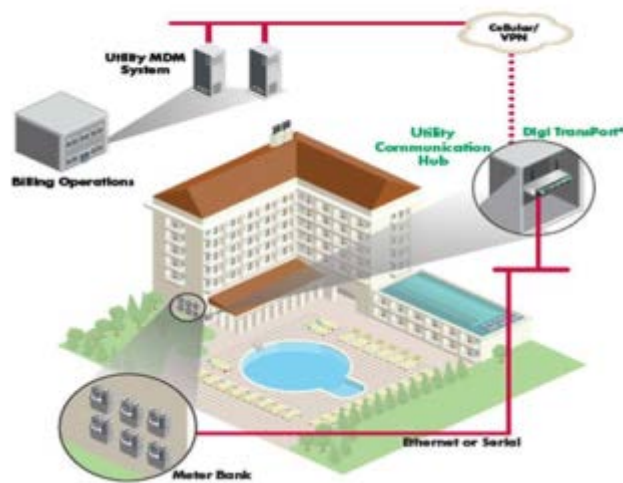
Figure A-34. Meter Remote Communication Diagram
