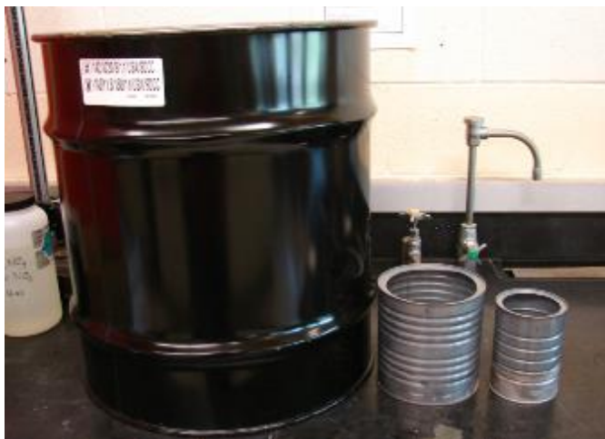
Figure 3-2. Three Test Systems Used in the Ionic Conductivity Feasibility Study (4-in. and 6-in. Diameter Cans and a 26-gal Container)
