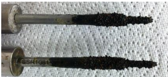
Figure D-2. Severe Corrosion on Tank TX-117 Specimen at +50 mV above Open Circuit Potential
