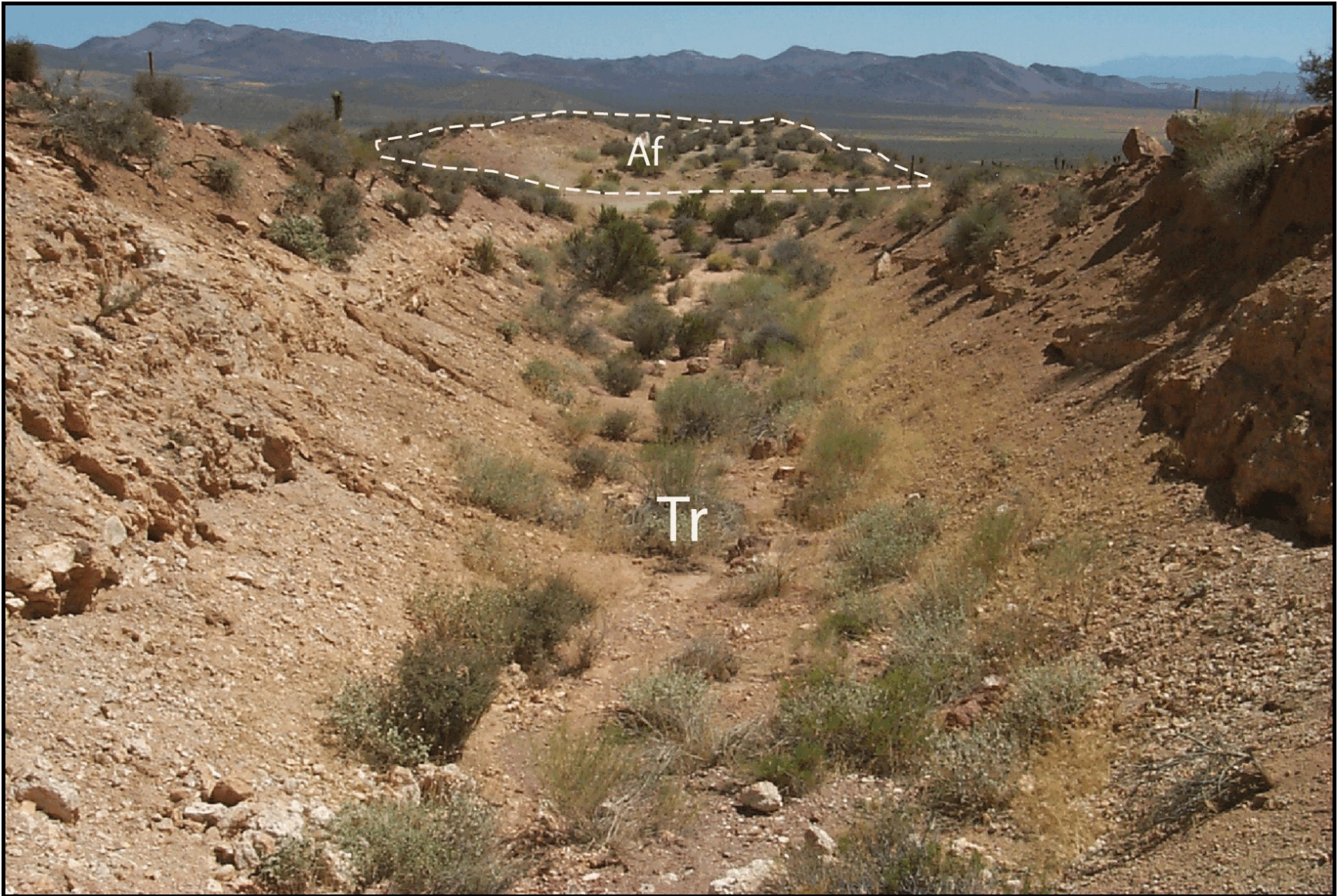
Figure 19. View south toward Yucca Flat of bulldozer trench excavated across the Boundary fault. Trench shows the resistant ledge formed of calcium carbonate, partially filled trench floor, and spoil pile (Af) derived from trench excavation.
