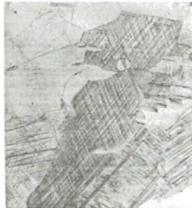
Fig. 13—Microstructure of annealed \alpha brass (21.40 wt % Zn) after 550-kbar shock. X250.
