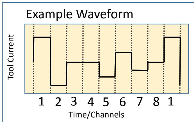
timing for eight channels in the frame. Take the center current reading for each channel; again channel 1 is marked as the highest amplitude and now all the reading can be recorded and saved as a frame.
