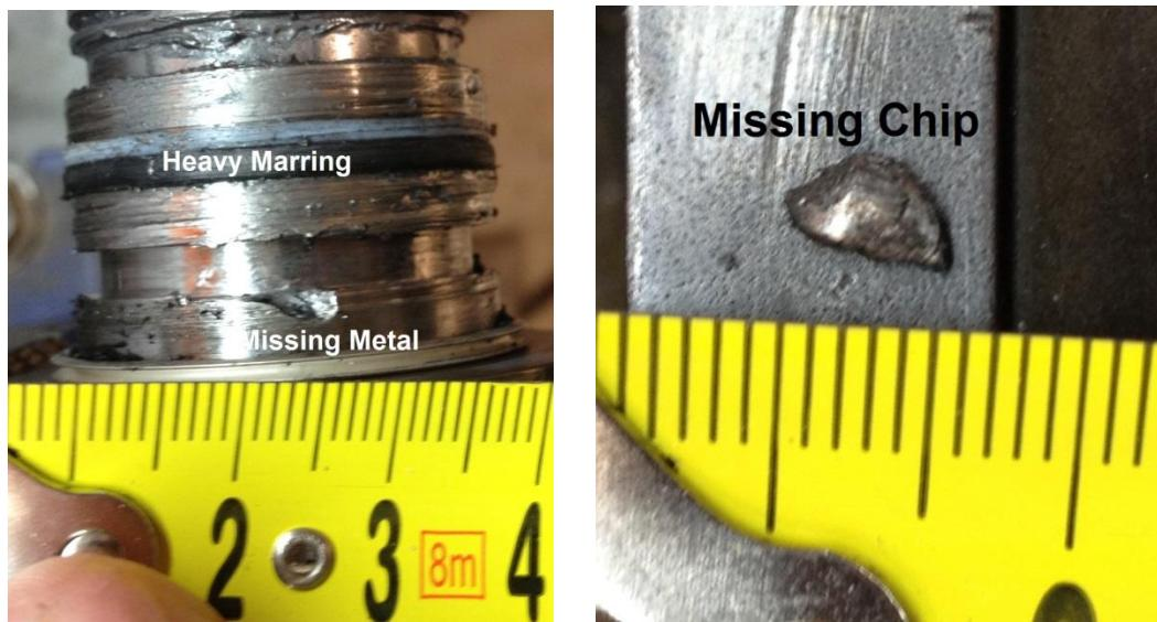
The image to the left is of the damaged O-ring groove. A large chip was actually broken out of the steel next to the O-ring groove. To the right is the missing chip.
