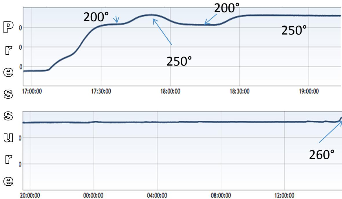
The downside to doing pressure only over such an extended time is that we do not have the corresponding temperature and P/T zero point data to help control drift or temperature related calibration changes.
