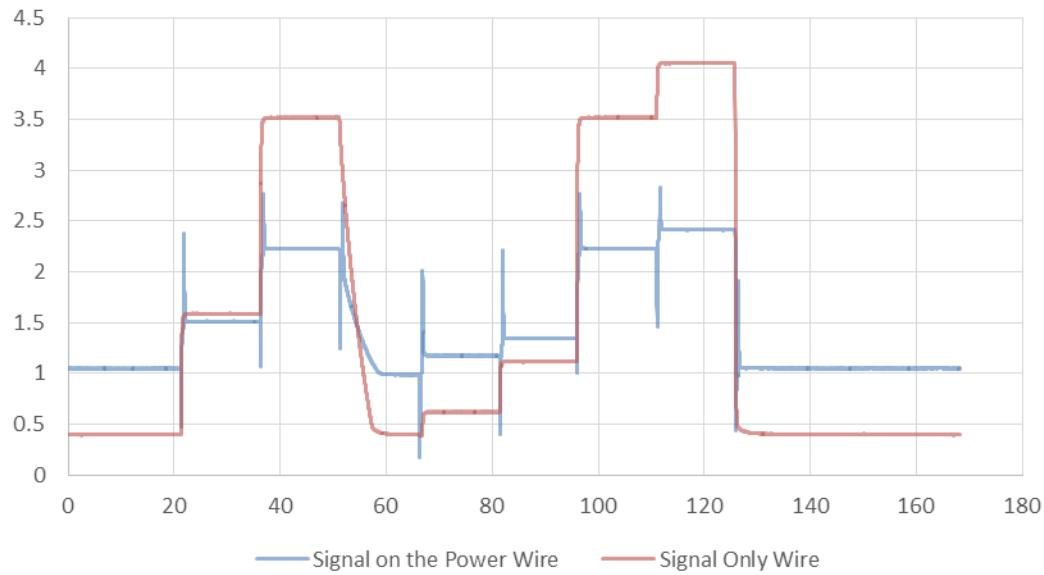
Also interesting in the above plot, the amplitude of the signal-only wire is much higher. This is true because the Perma Works tool has two-way communication. The surface communication to the tool is always on the power wire. To avoid conflicts, the surface communication to the tool is much larger and overrides the tool's PAM signal. Then, using a signal-only wire, the PAM signal is unbound.
