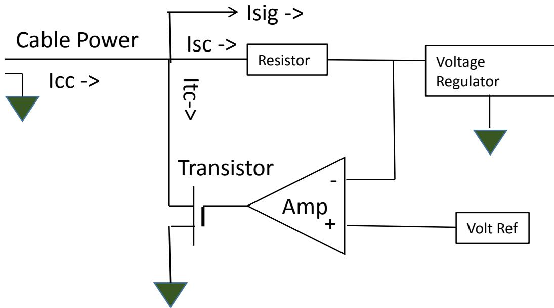
In the above circuit, the goal is to hold the supply current to the tool electronics to be constant even when the tool's supply voltage is changing. The current created by the sensors ( $Isig$ ) is allowed to change as needed. From above:
