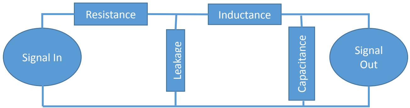
In the above cable loss model, the signal is subjected to a low pass filter. In short, the higher frequencies are attenuated more than low frequencies. The longer the cable, the more high frequency the attenuation. For geothermal well logging trucks, it generally assumed that the cable is 20,000 ft. long.
