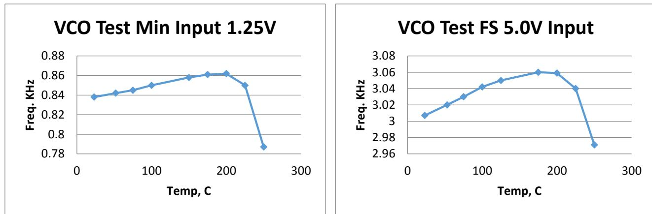
At higher temperatures, the frequency output is dropping. This creates an obvious problem; there are two output frequencies for every input voltage. The surface receiver could be confused when correction is made for temperature effects on the VCOs.
