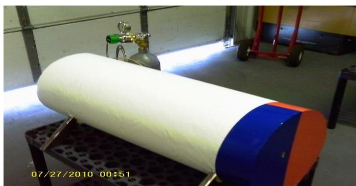
As free hydrogen in the geothermal well is always there and unstoppable, Perma Works has to test all electronic components for unwanted hydrogen effects using the hydrogen test chamber shown in the photo. Here, the round oven can heat electronics up to 400°C. The oven is completely sealed
