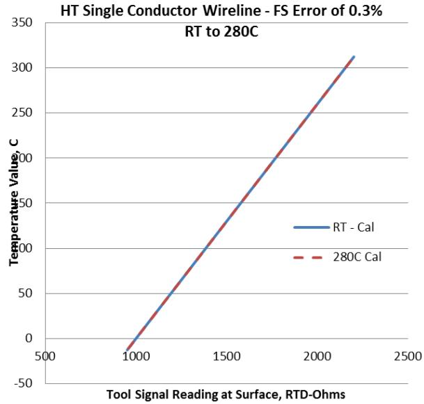
For these plots, the pressure sensor data (left) is in volts per Kpsi. The temperature sensor data is in ohms per degree C. In both cases, the room temperature plot sits on top of the 280°C plot. Even as the tool is rated to 275°C, testing is run to 280 °C. In fact, the tool electronics can be run to 300°C for short periods of time.
