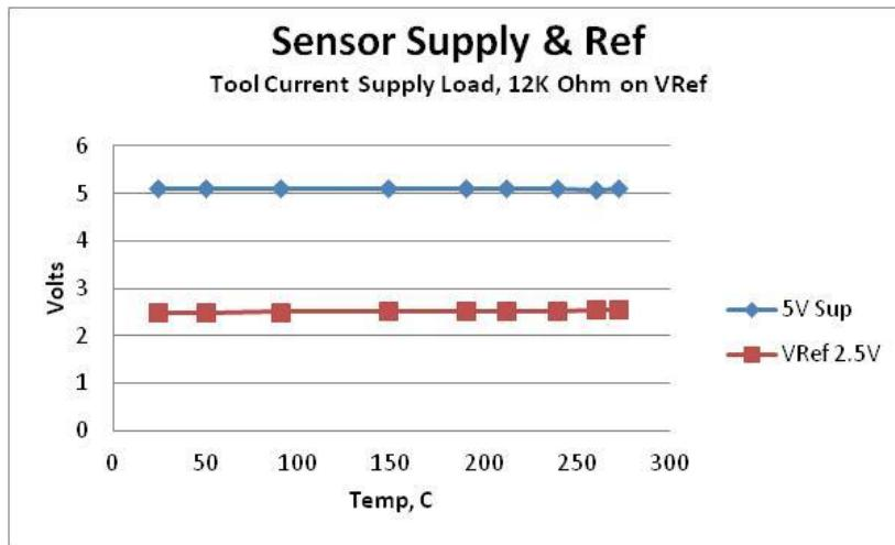
The plotted 5V DC tool supply and 2.5V reference voltage is shown to the left. The 5V supply is performing well with only an only a  $\sim$ 15mA load. This leaves room for adding other sensors in the future. The reference voltage started at 2.4948V and finished at 2.543V. The issue with the reference voltage is that any voltage change or noise on the voltage reference will also be seen on the sensor readings. A change of 48.2mV is significant.
