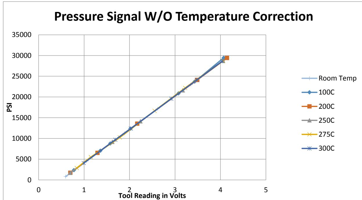
0.022V/30,000psi. That's only  $0.73 \times 10^{-6}$  V per psi. The geothermal reservoir engineer wants to track changes in the reservoir level within a few psi over a period of a year! So the question is how to best get this signal to the surface with most accuracy and best signal to noise ratio?
