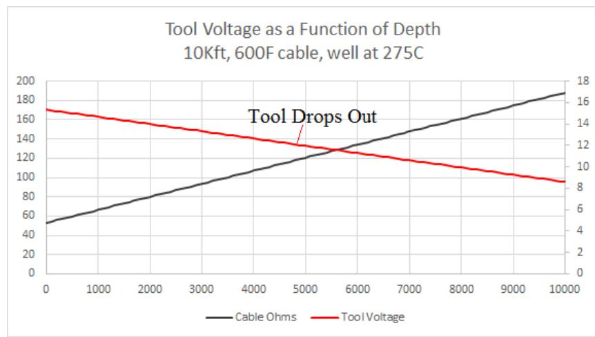
In the plot below, when the cable head voltage falls to the tool's minimum operating voltage of 12V, the supply voltage at the truck is increased. This happens at the
