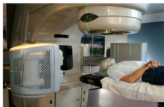
Figure 7: The Varian Medical System for treating a patient with x-ray produced by a high-energy electron beam.
