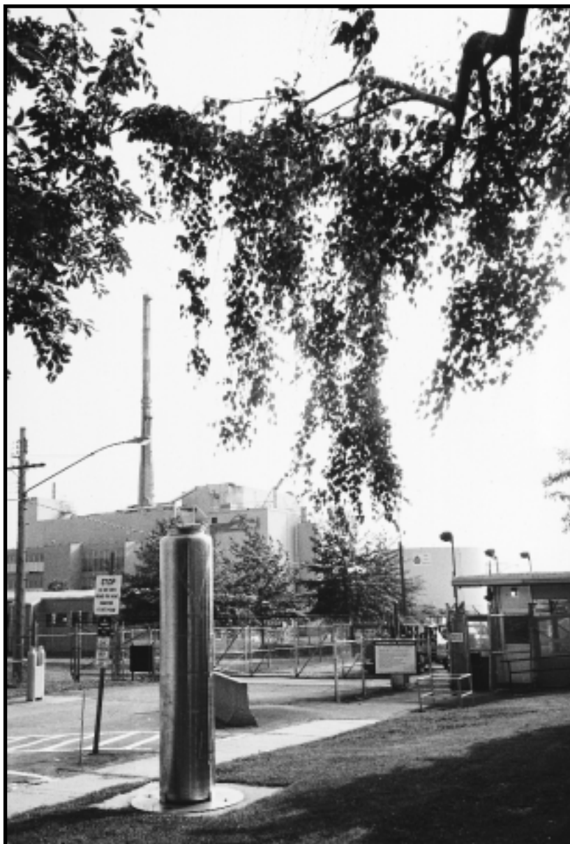
Stainless Steel Canister for Vitrified Waste at West Valley Demonstration Project. This 10-foot by 2-foot stainless steel canister is identical to those being used to store vitrified high level radioactive waste prior to disposal in the proposed geologic repository. The waste, primarily cesium-137 and strontium-90, was generated from reprocessing commercial spent nuclear fuel to recover uranium and plutonium and was stored in a 740,000-gallon tank. Vitrification of the liquid high-level waste (containing most of the cesium-137) was completed in June 1998. DOE is now removing and vitrifying the “tank heel,” the remaining sludge layer at the bottom of the tank, which contains most of the strontium-90 and transuranic elements. West Valley Demonstration Project, New York, June 1999.
