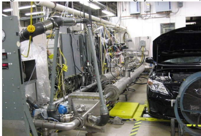
Figure 9-3 Vehicle during FTP driving cycle (side view)
