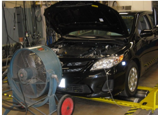
Figure 9-2 Vehicle during FTP driving cycle (front view)
