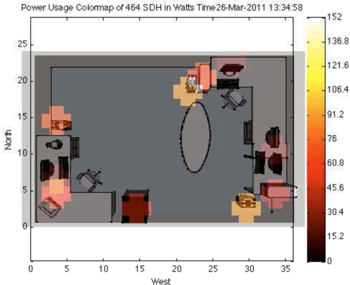
Figure 87: Display of the floor plan of test lab in Sutardja Dai Hall, colors over appliances represent real-time power draw.
