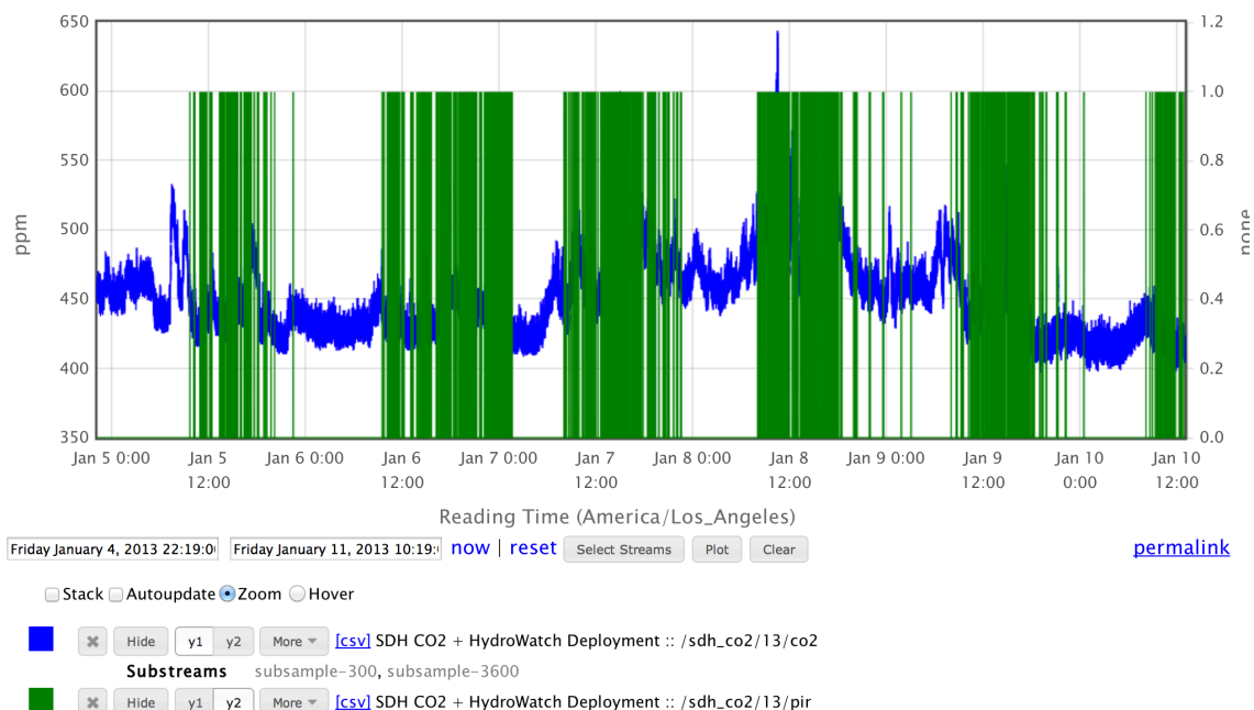
Figure 110: CO 2 (blue) and motion sensor (green) values in one bay of a cleanroom. Identifying periods of inactivity will allow energy savings by turning down the rates of recirculating air handler units (RAHUs).
