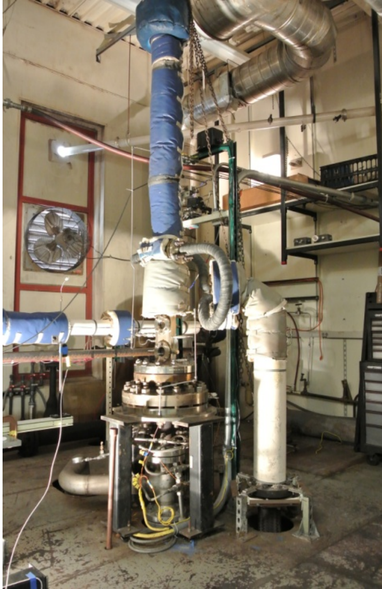
Figure 4-1: Flameholder test stand in the UC Irvine High Pressure Combustion Facility
