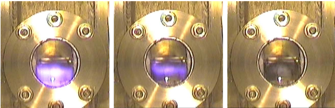
Figure 5-3: Blow off sequence for a natural gas flame with the reverse step
