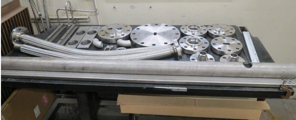
Figure 4-4: Flameholder test rig components prior to assembly
