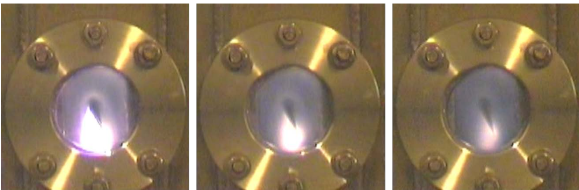
Figure 5-4: Blow off sequence for a natural gas flame with the rotated airfoil
