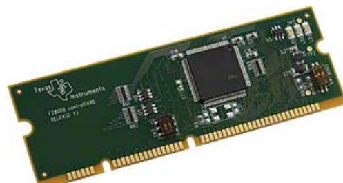
EVAL KIT FOR TMS320F28X (TMS320F28069)
