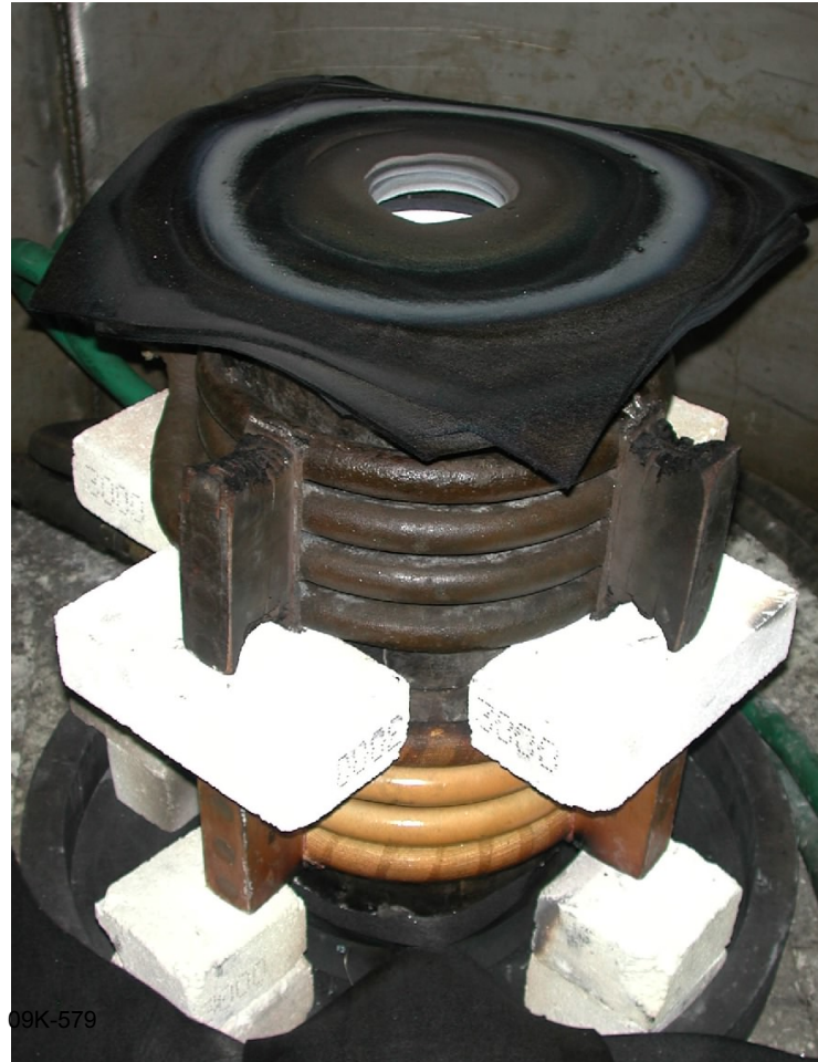
Mold stack with 12" diameter induction coils for mold heating and insulation
