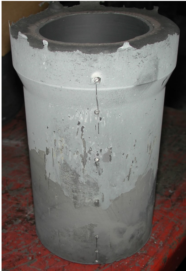
Casting just after removal from mold. Thermocouple remnants and residual mold coating can be seen.
