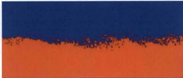
Cu(2D) P=30\text{GPa} , v=0.12c_s , Mechanical Mixing
