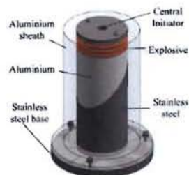
Figure 2. The FN0 experiment. The aluminium (top) and stainless steel (bottom) components were machined to a surface roughness of \lambda/2\mu\text{m} and were flat such that the maximum gap that could exist between the sliding surfaces was <25\mu\text{m} . The components were held in contact by gravity.
