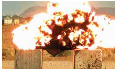
Explosive test on a door panel conducted at Sandia National Laboratories
