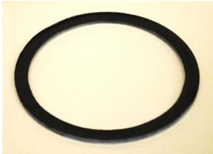
Figure 4.1: A 1/10th scale model toroid casting of iron particles 40 vol.% in custom epoxy formulation.
