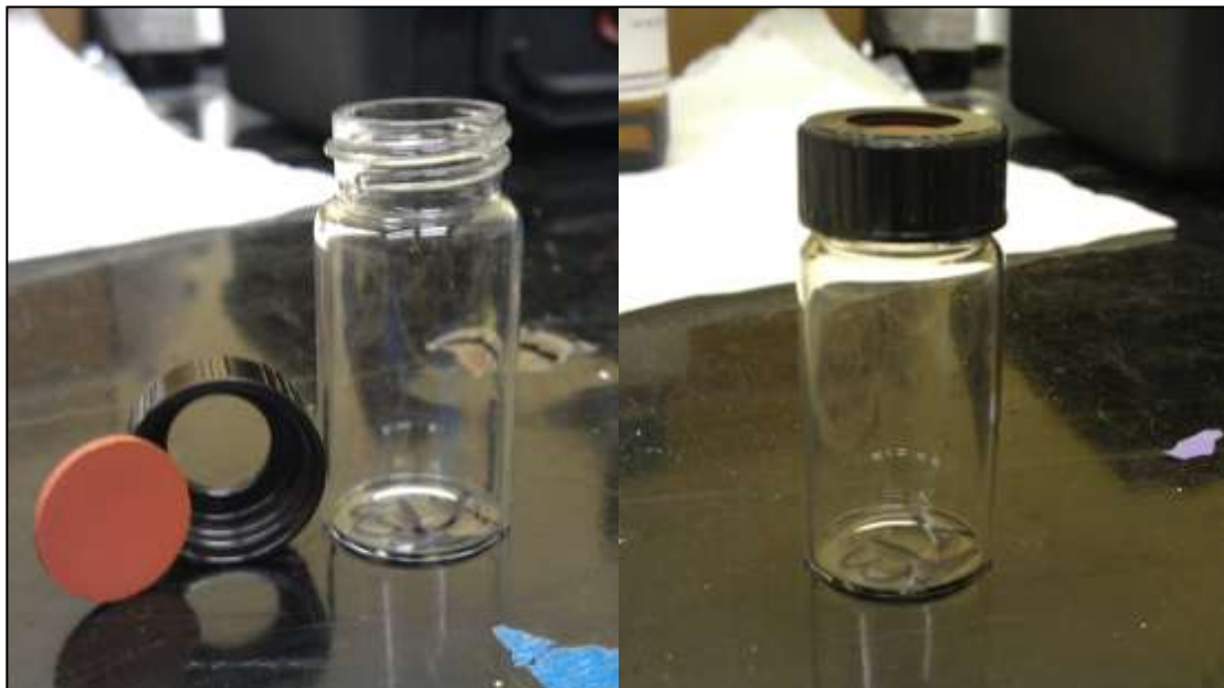
Figure 1: Emission vial for PFT sources. The photo on the left shows the vial cap and rubber septa insert separated. The photo on the right shows the assembled vial with septa inserted into the vial cap.
