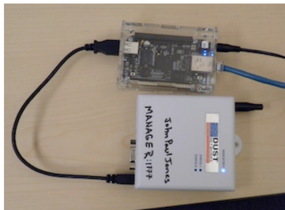
Figure 4. Manager mote and embedded computer.
