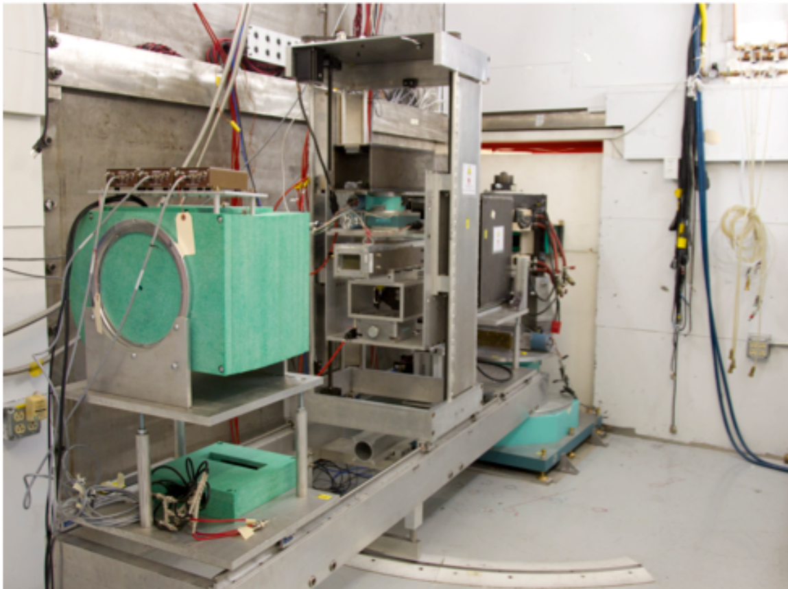
Figure 2. Photograph of the new secondary spectrometer installed on Asterix as part of this project.
