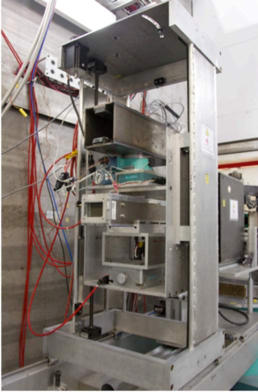
Figure 4: Left: more detailed view of the elevator that allows two different polarization analyzers and an empty beam pipe to be placed in the neutron beam. The 2 polarization analyzers are (from the top): a single-supermirror polarization analyzer with new mirrors purchased as part of this project and a wide-angle polarization analyzer obtained from the IPNS. Figure 4: Right: Close up view of the new detector housing mounted on the secondary spectrometer gantry. One of the detectors that is not in use is seen on the shelf below the main detector housing.
