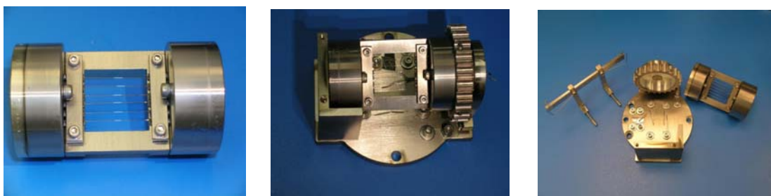
Fig. 14: Components of fiber sputter coating jig. (Left) hanger; (center) carrier plate and rotation wheel; and (right) fiber holder drum. Wire clips on carrier plate hold flat substrates used as witness samples to measure metal thickness.
