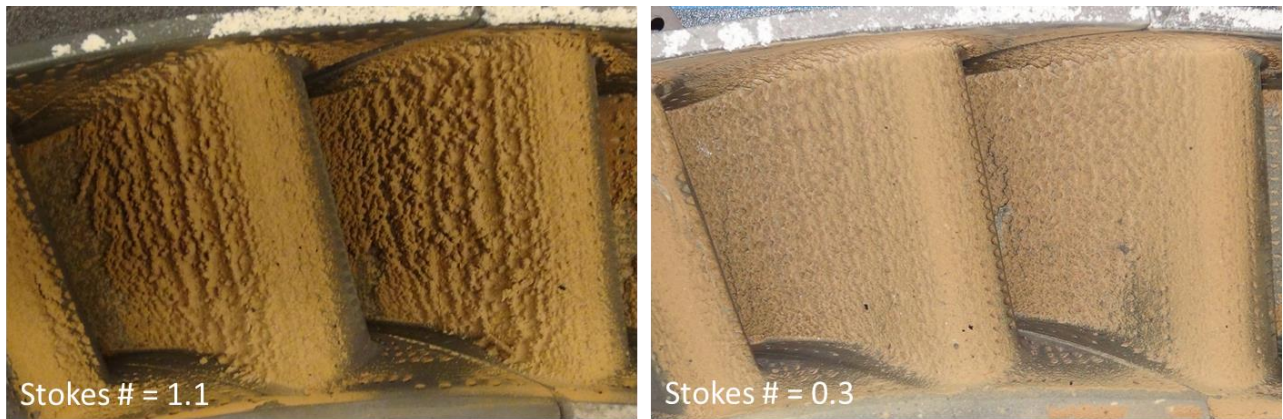
Figure 43: Deposits on CFM56 vanes for different Stokes numbers
