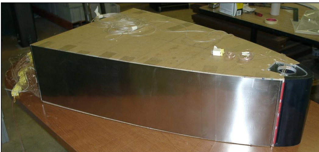
Figure 16. Photo of smaller film cooling cylindrical leading edge test surface.
