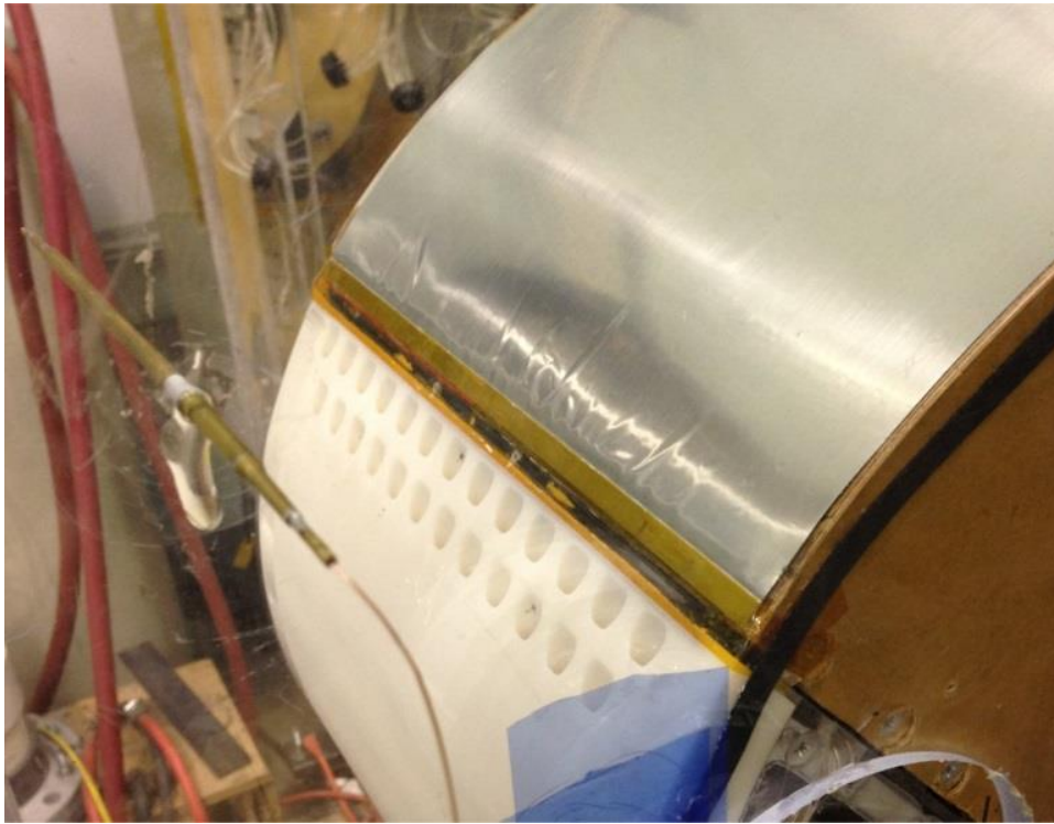
Figure 20. Photo of shaped hole insert installed onto cylinder upstream of bracket instrumentation and heat transfer foil.
