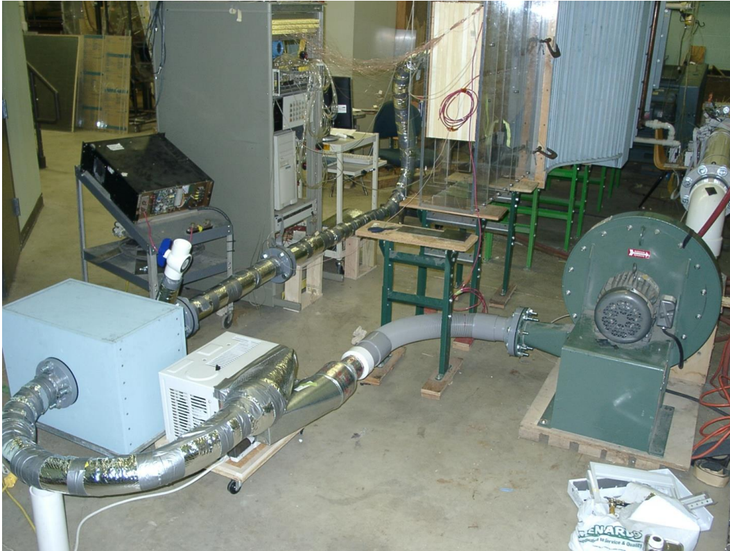
Figure 13. Film Cooling Air Delivery System Showing Blower, AC Unit, Thermal Capacitance Unit and Orifice Tube.
