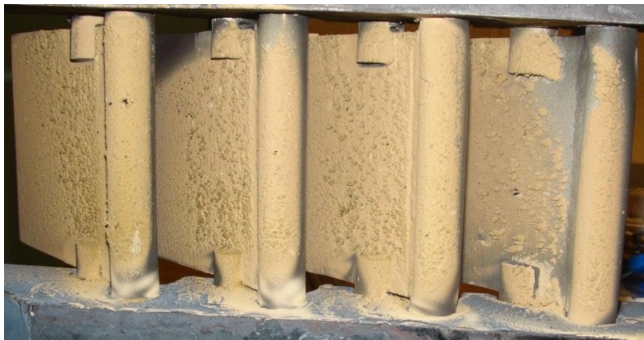
Figure 38: Post test image of 0.5" diameter cylinders with deposition intact. Internal cooling was used to limit thermal expansion.
