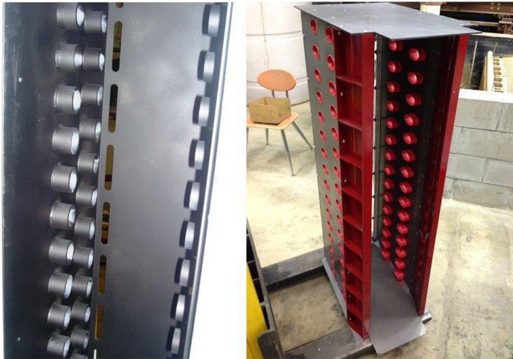
Figure 22. Comparison of old and new very high turbulence aero-combustor simulator.
