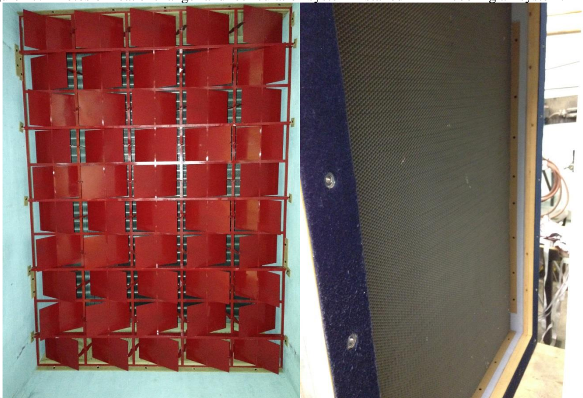
Figure 27. Photos of heat exchanger and recirculation system installed in film cooling air system.
