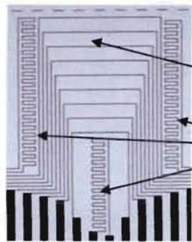
9 Particle Velocity ( $u_p$ )3 Shock Trackers ( $U_s$ )
