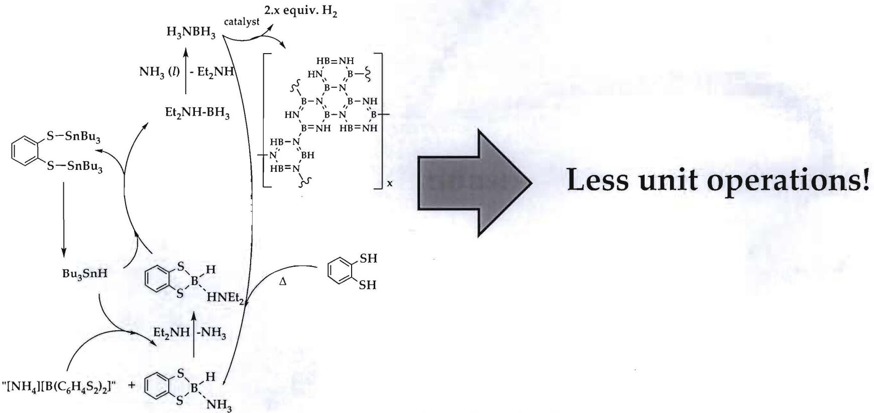
e.g. Less  $C_6H_4(SH)_2$  in digestion = less Sn-H required = minimize recycle!
