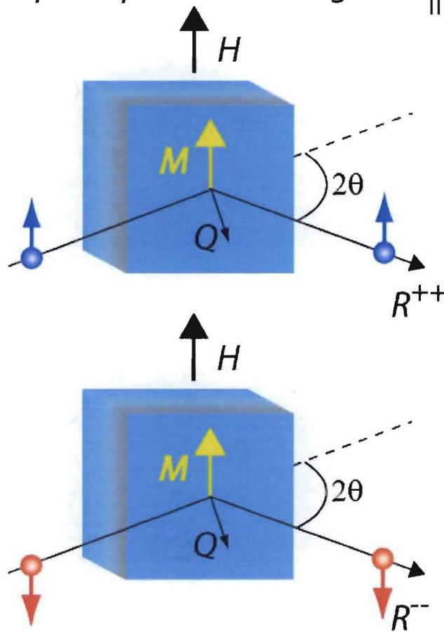
Measurement of the neutron scattering as a function of wavevector transfer (of order  $0.1 \text{ \AA}^{-1}$ ) allows us to determine the structures and properties of materials that are non-uniform with nanometer resolution.
