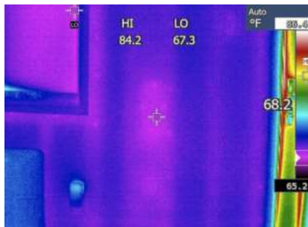
Figure 7 - P1 thermal bridge at deck support bracket
