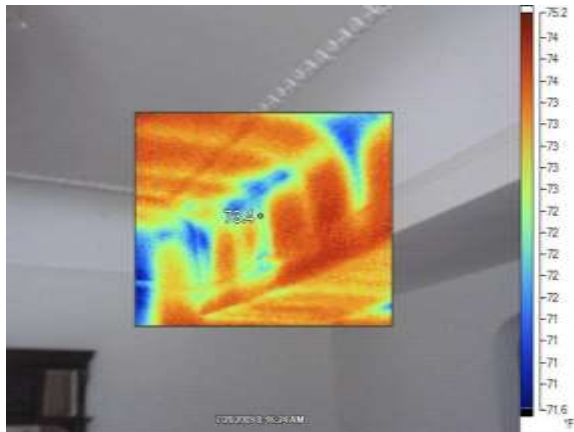
Figure 107 - P7 Pre-retrofit thermal leakage in master bedroom
