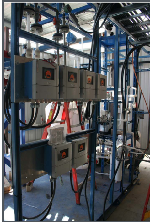
Figure 6. Control system of lithium hydroxide pilot at Simbol's Brawley, CA facility.
