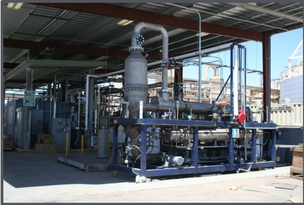
Figure 4. Simbol's lithium extraction pilot plant Calipatria, CA adjacent to CalEnergy's Elmore geothermal power plant.
