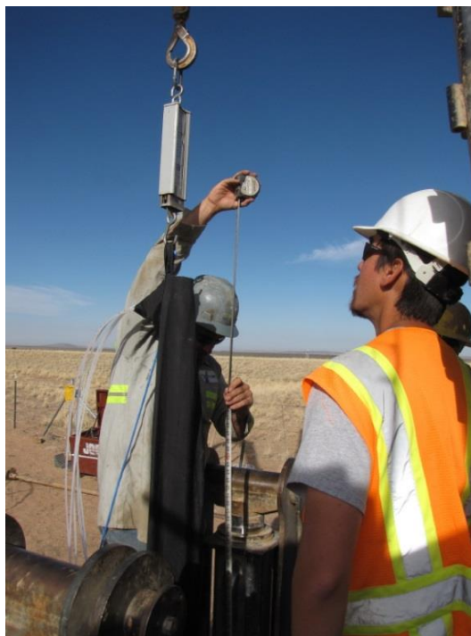
Figure F-6 Use of weight scale to verify that FLUTe™ borehole liner is deployed to the proper depth in the drive casing prior to inserting the tremie pipe at soil-vapor monitoring well MWL-SV04.
