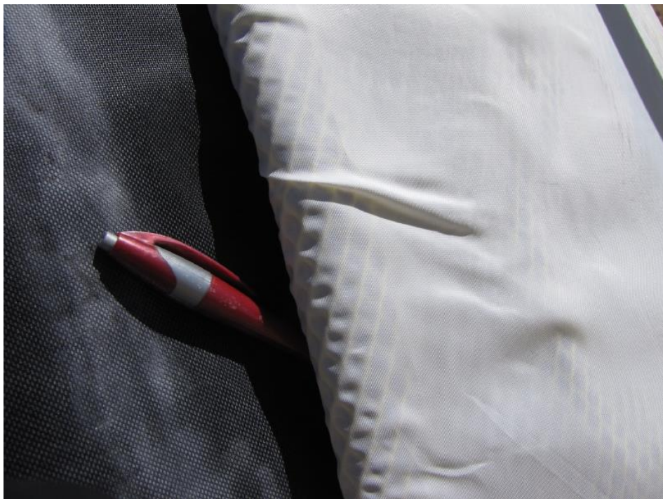
Figure F-4 One of five permeable spacers for soil-vapor monitoring well MWL-SV03. The outer permeable fabric (white) covers the diamond mesh. The impermeable borehole liner is the black fabric.
