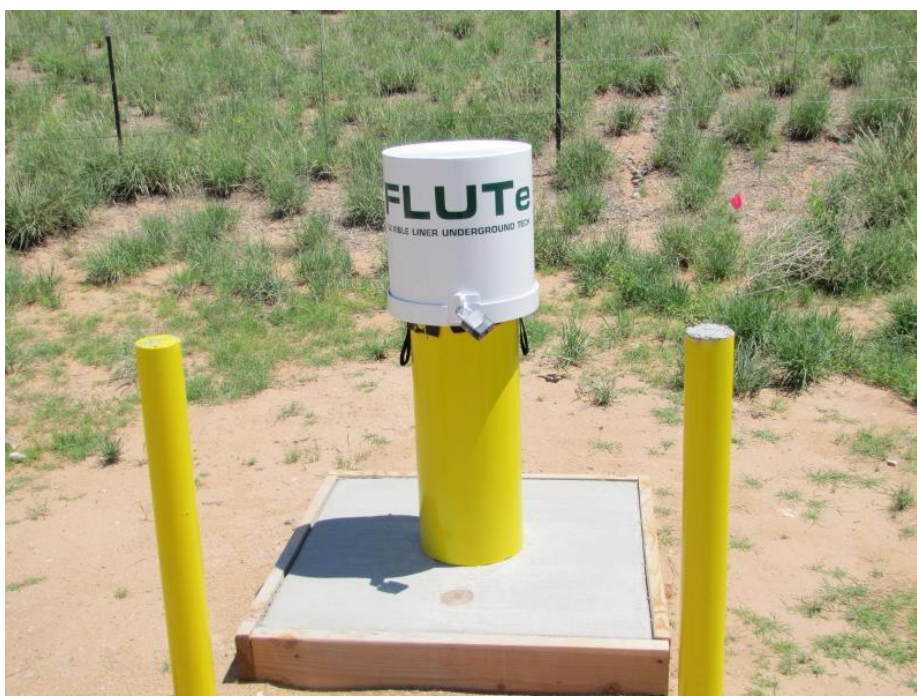
Figure F-14 Completed installation for soil-vapor monitoring well MWL-SV03.
