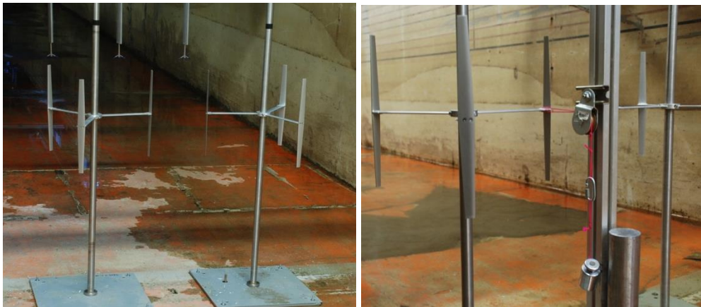
Figure 3: Photos of the RM2 dual-rotor model in the SAFL Main Channel (left) and during torque sensor calibration (right) performed by applying known forces to the rotor and torque sensor.
