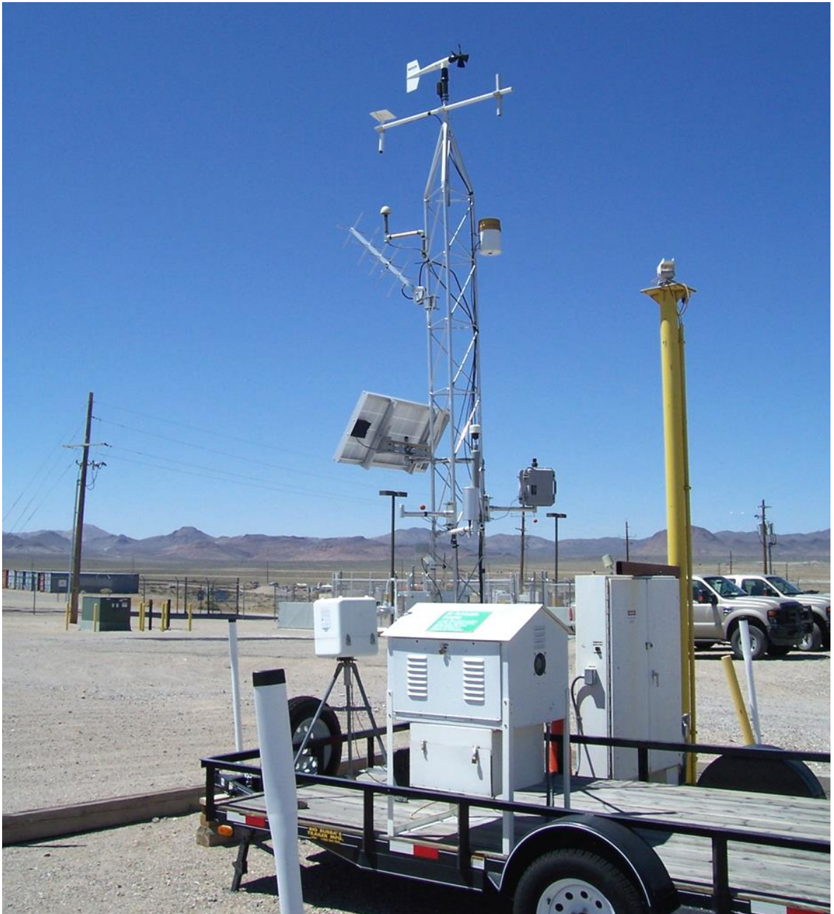
FIGURE 1-3. Station 400 measures radiological and meteorological conditions near the Range Operations Center (ROC) in the Sandia National Laboratories compound on the Tonopah Test Range.
