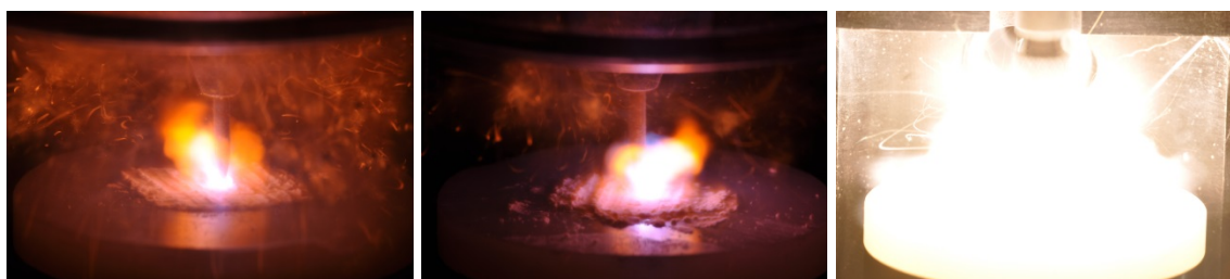
Figure 3. Positive reactions of sugar (52.9%, 1.25J), sawdust (44.2%, 1.25J), and Al (26.5%, 0.025J) mixtures
