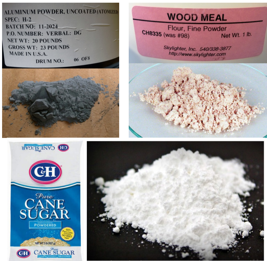
Figure 2. Aluminum, sawdust/wood meal, and powdered sugar fuels
