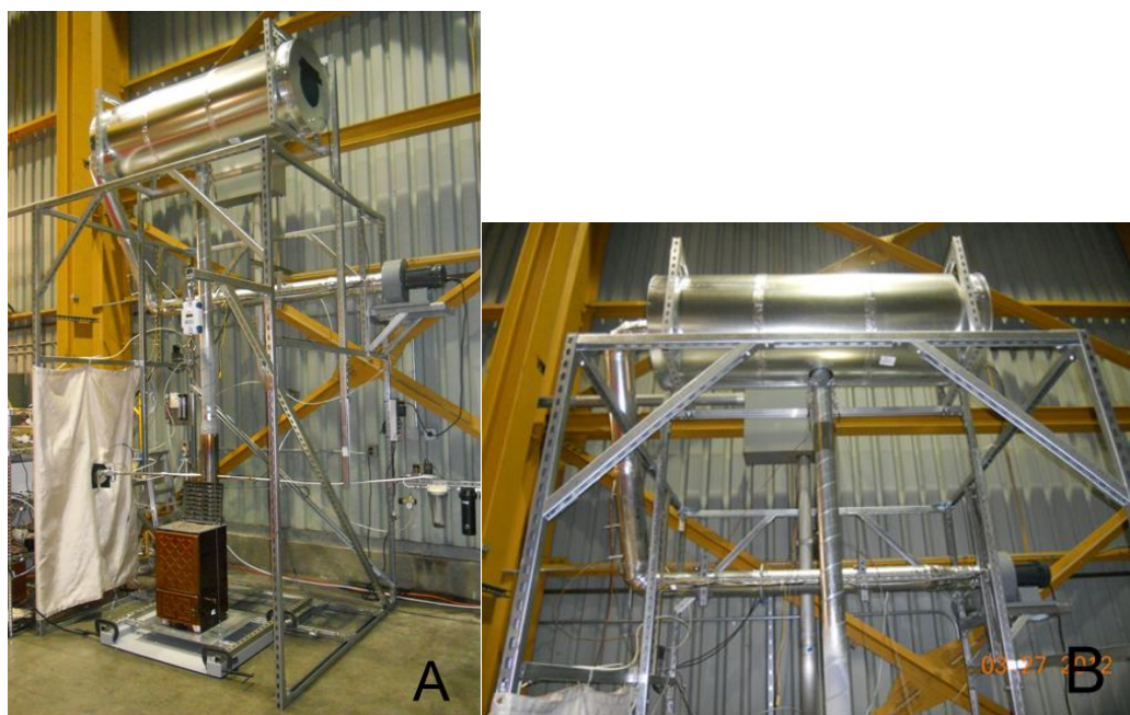
Figure 1: Panel A shows the complete system including stove mounted over a weight cell with chimney extended into the exhaust dilution tunnel then ducted down behind the apparatus to a ventilating exhauster. Panel B shows the detail of the upper dilution tunnel and exhaust ventilation ducting system. The instrumentation rack is mounted to the left behind the fire curtain and the particle free dry air is generated by a compressor mounted to the right of the system (not shown).
