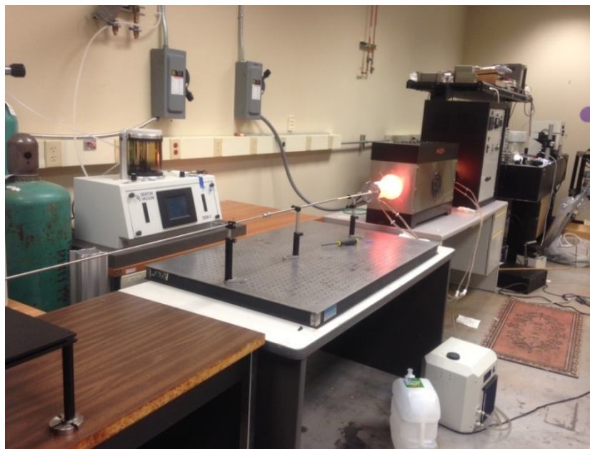
Figure 22-4. Fully packaged sapphire fiber sensor inserted into a hot furnace. The sapphire sensor showing is the longest sensor for the purpose of in situ monitoring of the gasification process (to be inserted from the top). Other sensors with shorter lengths are being constructed for monitoring other power systems such as a gas turbine.
