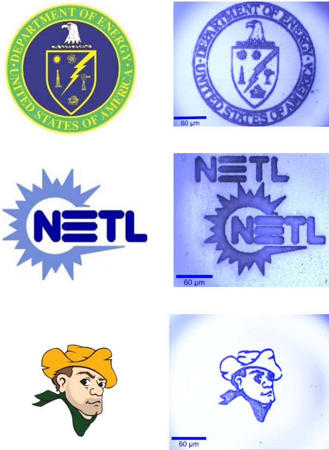
Figure 3-3. Microscopic images of example patterns fabricated on sapphire substrates using the developed femtosecond laser micromachining system. The direct ablation is facilitated by air-blowing to remove debris. The smallest features that can be achieved is about 1\mu\text{m} in width.
