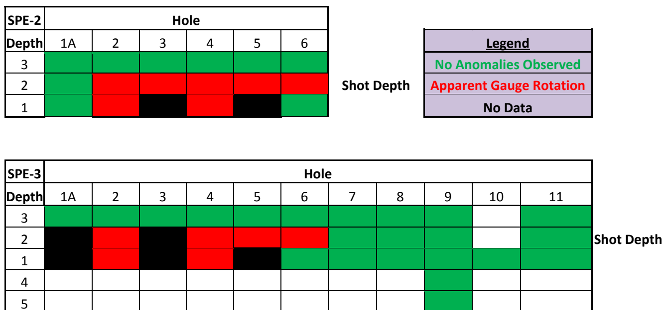
Figure 18: Figure 19: Stop light chart summarizing data for SPE-2 and SPE-3 including new gauge canisters.
