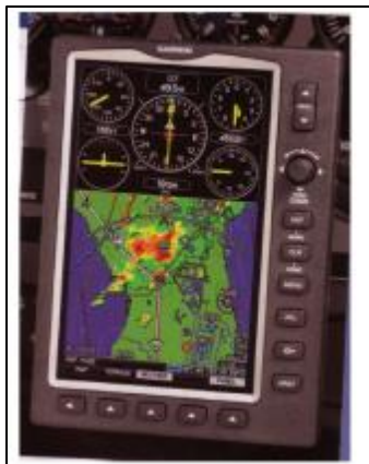
FIGURE 13 GARMIN 696 NAVIGATION UNIT AS USED BY NRCAN BY THE PILOT FOR SURVEY NAVIGATION.
