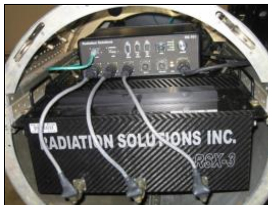
FIGURE 4 THE RS-701 CONSOLE ON TOP OF THE RSX-3 DETECTOR BOX.
