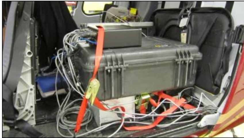
FIGURE 12 INTERNALLY MOUNTED EQUIPMENT: ON THE BOTTOM TWO RSX-1 CRYSTALS AND RSN-4 NEUTRON DETECTOR; ABOVE THAT, THE BATTERY BOX AND POWER DISTRIBUTION SYSTEM WITH RS-705 CONSOLE ON TOP. THE POWER DISTRIBUTION SYSTEM AND CONTROLLING LAPTOP ARE BARELY VISIBLE BEHIND THE BATTERY BOX AND CONSOLE. EQUIPMENT WAS STRAPPED TO TIE DOWNS IN THE AIRCRAFT.
