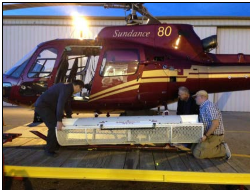
FIGURE 10 INSTALLATION OF THE NRCAN SYSTEM ON THE SUNDANCE AS350 HELICOPTER.
