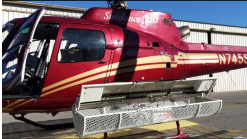
FIGURE 11 NRCAN BASKET WITH RSI DETECTORS MOUNTED TO THE AS350.
