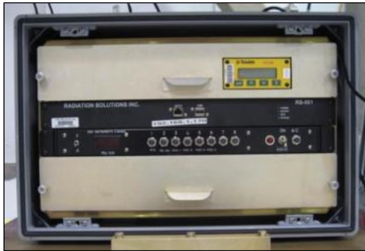
FIGURE 5 RS-501 AGGREGATOR CONSOLE WITH THE TRIMBLE GPS RECEIVER.
