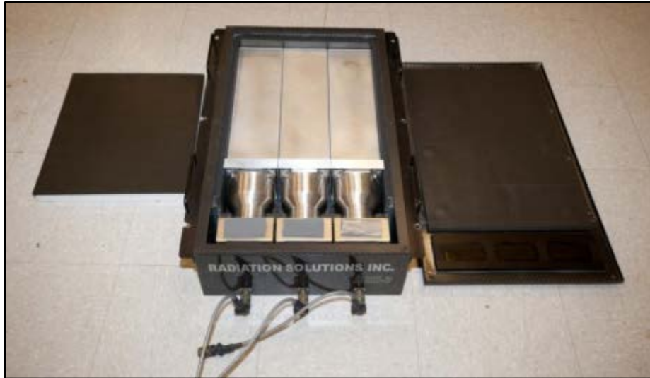
FIGURE 3 RSX-3 BOX WITH THREE 2" × 4" × 16" NAI(TL) CRYSTALS.
