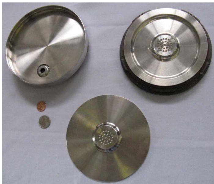
Figure 8. Lower surfaces of the Hagan, SAVY-4000 and NFT filter standard (clockwise from upper left).
