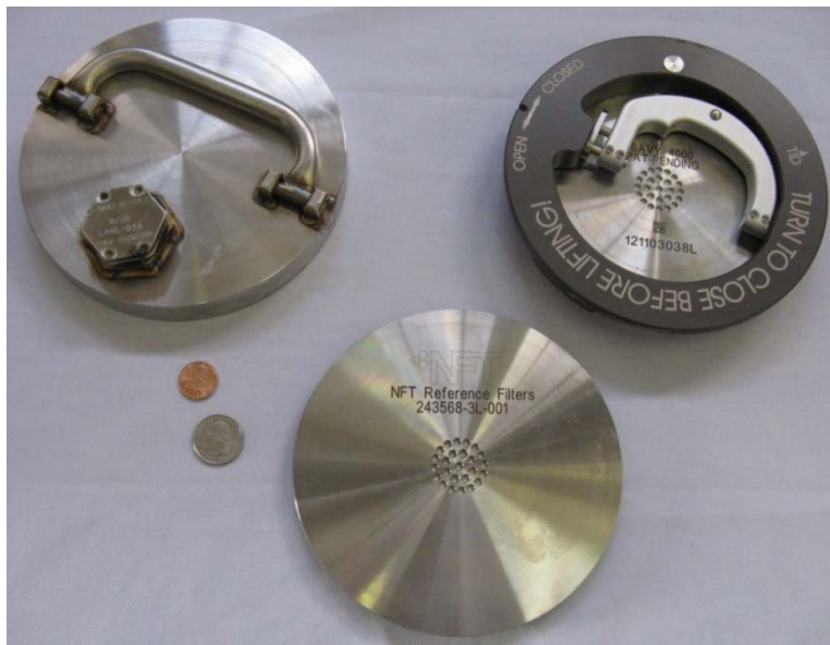
Figure 7. Top surfaces of the Hagan, SAVY-4000 and NFT filter standard (clockwise from upper left).
