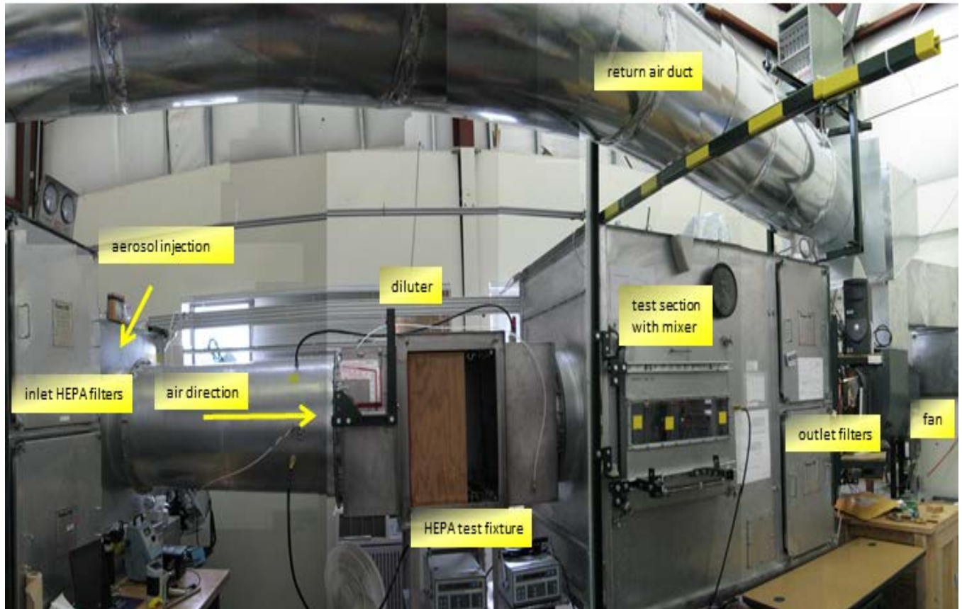
Figure 1. The Los Alamos aerosol wind tunnel requires completion and integration of three systems (i.e. mixer, diluter and performance-based air flow measurement).
