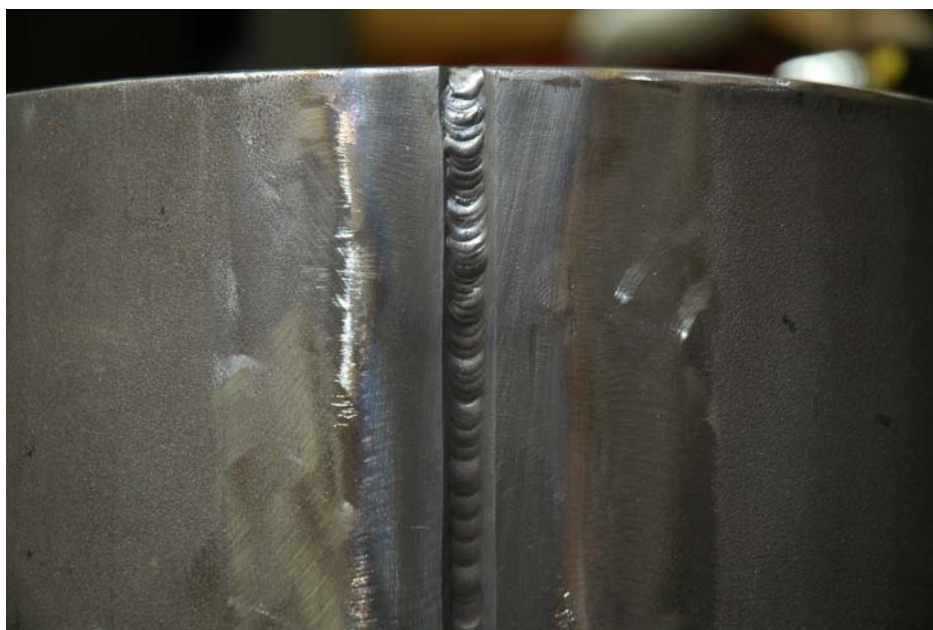
Figure 3.6: The root pass of the nickel purification vessel.
