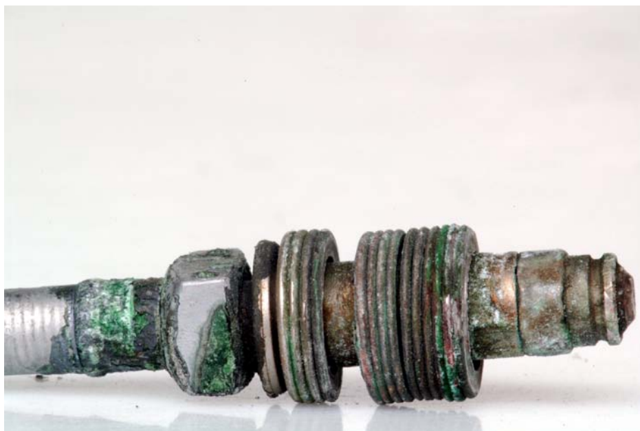
Figure 4.1: Failure of the bellows and the valve stem.
