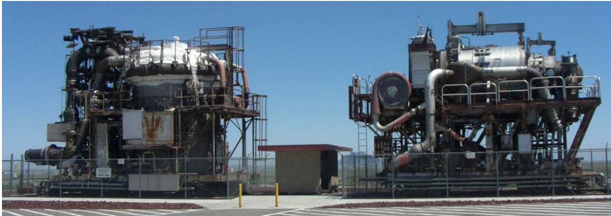
Figure 1.1: The two of the experimental reactors used for the ARE. The Heat Transfer Reactor Experiment 1 (HTRE-1) is on the right, the HTRE-3 on the left.
