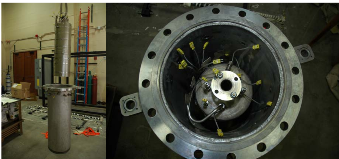
(a) Lifting the purification vessel into position
