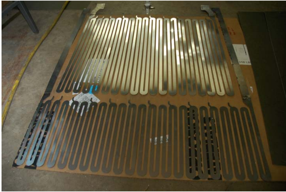
Figure 3.17: Two zone serpentine heaters with resistances around 3.2\ \Omega and 2.0\ \Omega producing a total 3000 W.
