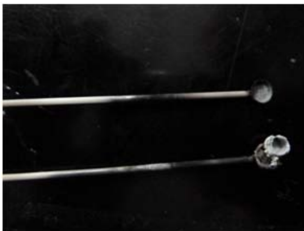
Figure 5.1: Creep of heated salts from the Seiko sample pans and fusing/corrosion of sample pans.
