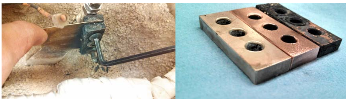
(a) The rabbit ear-copper block heater connectors. (b) Three states of the copper blocks. From left to right: Silver coated, polished copper, heavily oxidized copper.
