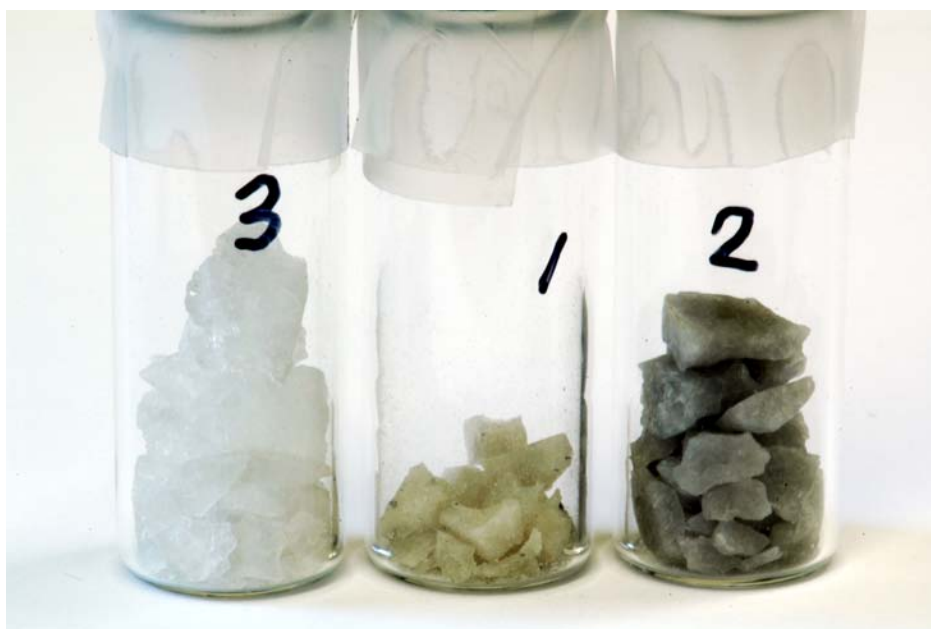
Figure 4.9: A comparison of University of Wisconsin flibe and MSRE flibe. From left to right: re-purified MSRE flibe, salt melted in open atmosphere from raw components, salt melted in a glove box from raw components.
