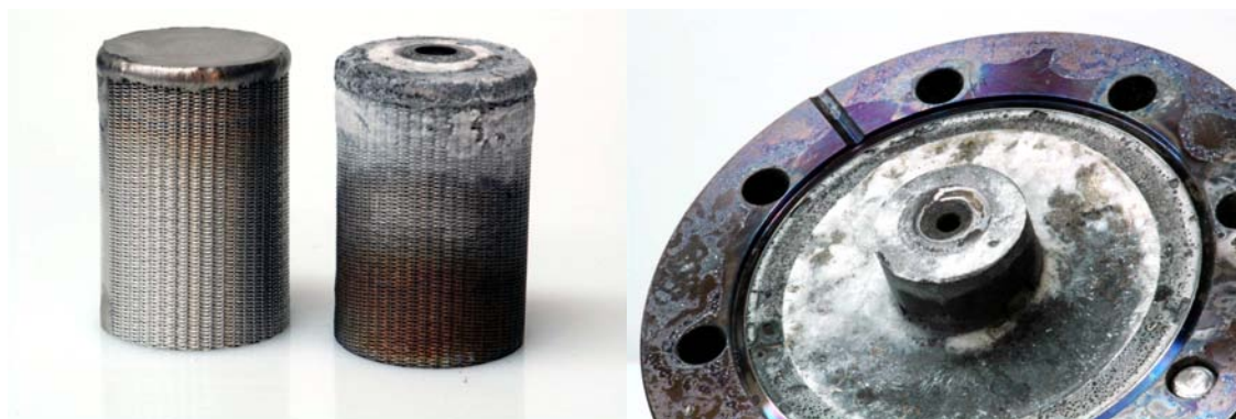
(a) A comparison of the filter unit before(left) and(b) The lid the filter unit showing a large buildup of \text{ZrF}_4 snow.
