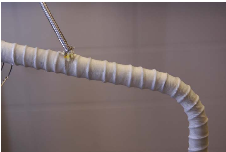
Figure 3.19: Finished, uninsulated trace heat. The top left shows a welded on thermocouple.
