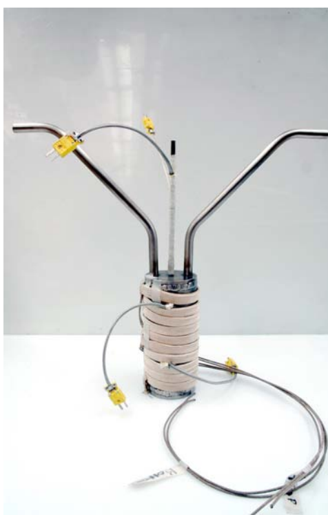
Figure 3.8: The small nickel purification vessel used for the purification of the MSRE flibe.
