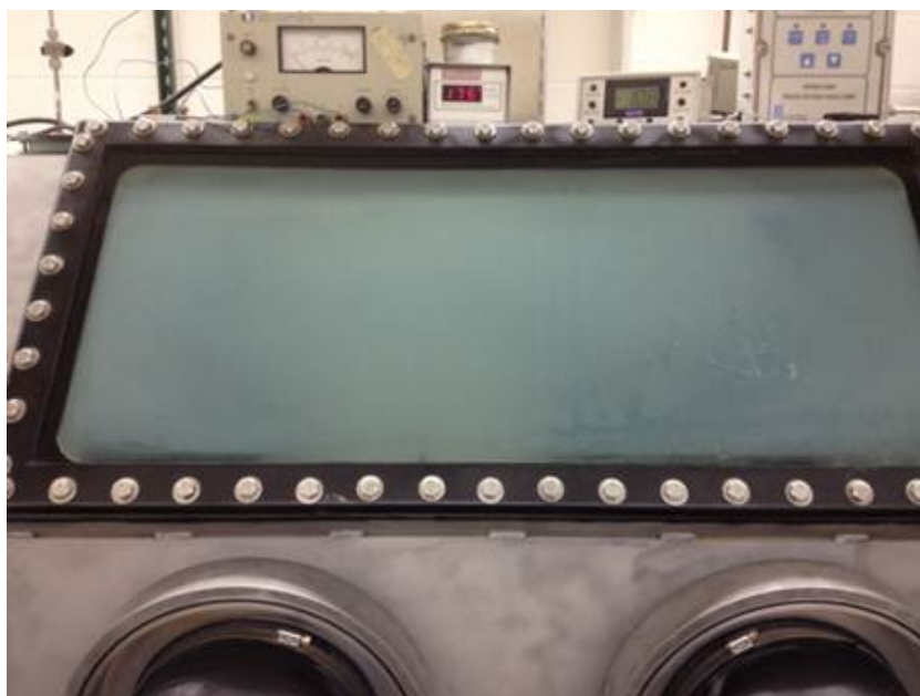
Figure 2.13: A glovebox used for melting zirconium fluoride salt with unknown amounts of water. The windows were etched by hydrogen fluoride vapor.
