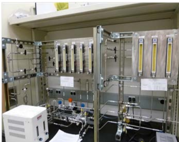
Figure 5.2: Dual manifold for gas delivery to vacuum line: NF 3 , F 2 , HF, ClF 3 , H 2 , O 2 , Ar, He.
