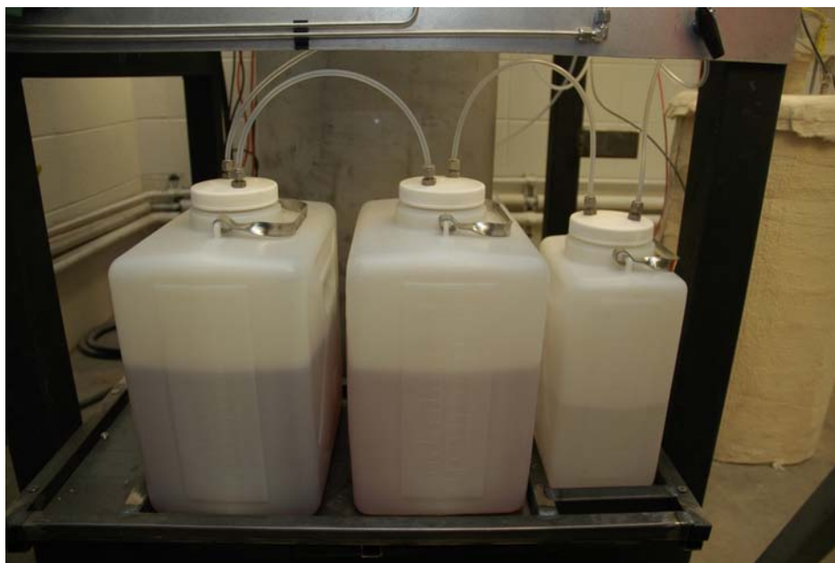
Figure 3.12: The carboy system for removing unwanted hydrogen fluoride.
