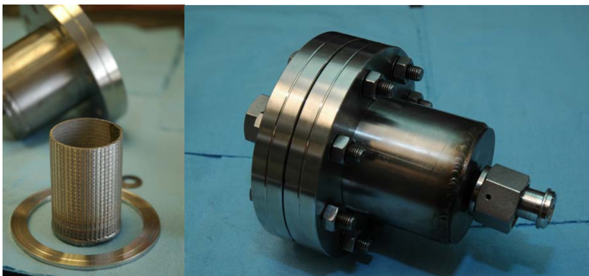
(a) The porous metal filter and other disassembled components
