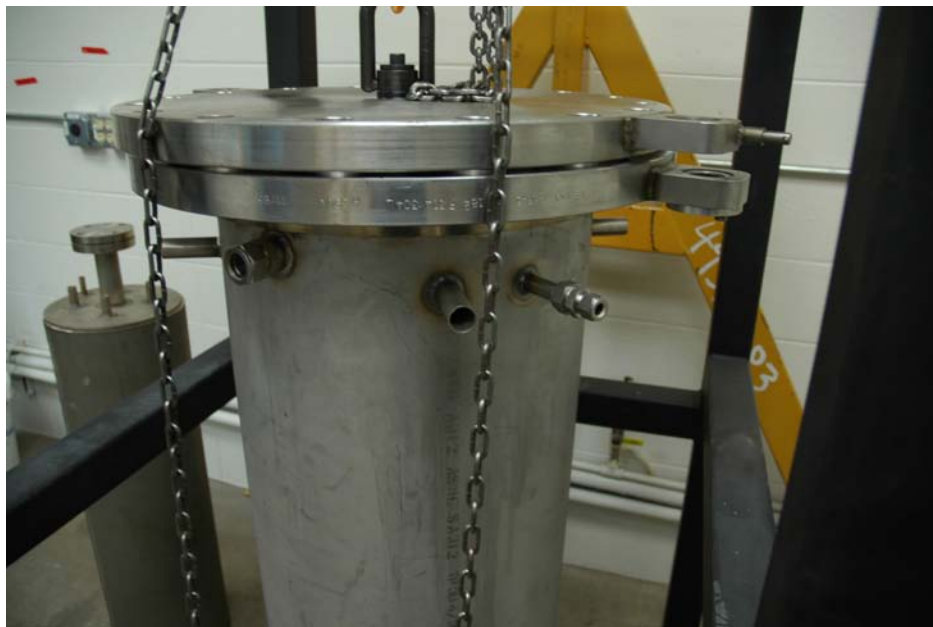
Figure 3.9: The stainless steel support vessel with the nickel purification vessel in the background for comparison.
