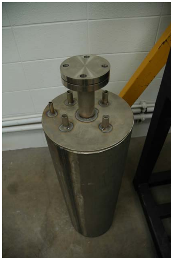
Figure 3.7: The nearly completed nickel purification vessel.
