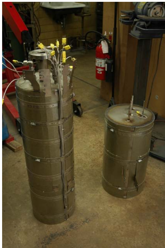
Figure 3.18: The purification vessel and the receiving vessel with mica and heaters attached. Thermocouples have been welded on at this point.
