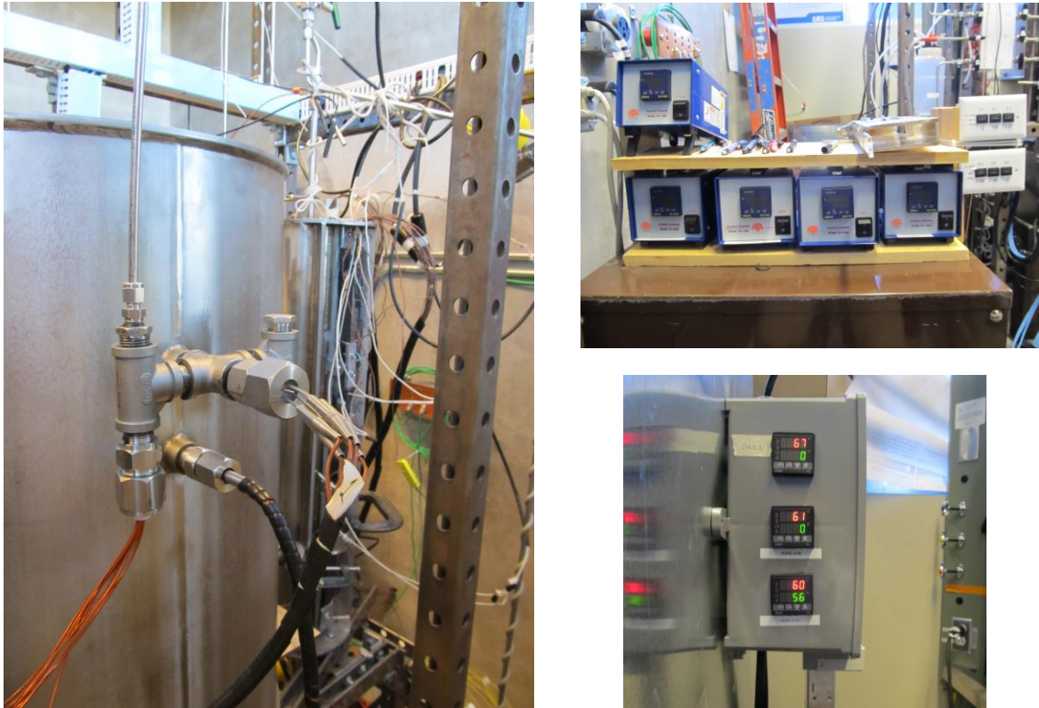
Figure 3.5. Thermocouple Penetrations on Instrumentation Tank and temperature controllers
