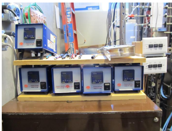
Picture 9a and 8b. (a) Temperature and valve control station for components external to the instrumentation tank. (b) Temperature control station for components internal to the instrumentation tank
