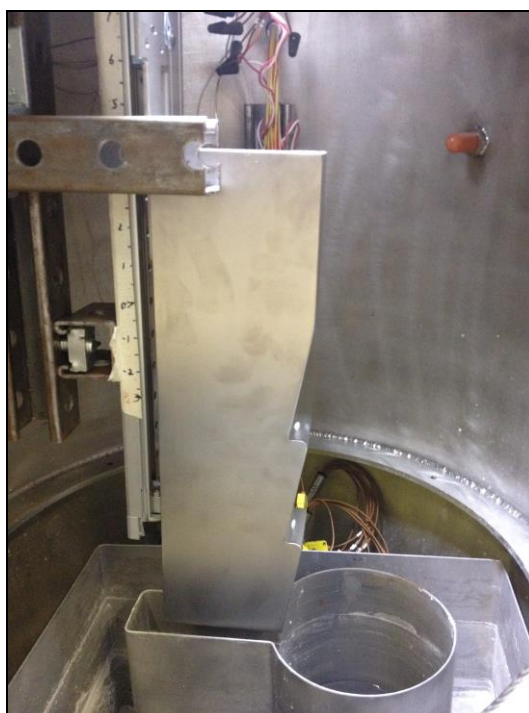
Figure 3.7. Transducer Cooling Jacket on Linear Actuator
