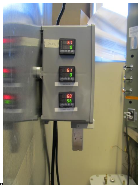
Picture 9a and 8b. (a) Temperature and valve control station for components external to the instrumentation tank. (b) Temperature control station for components internal to the instrumentation tank
