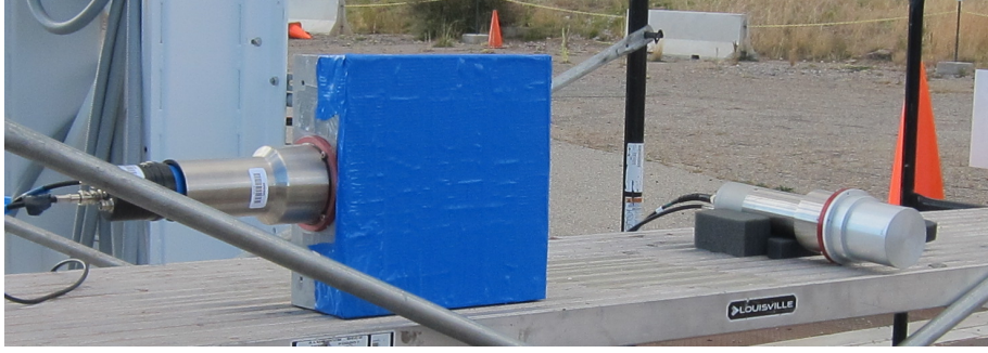
Figure 1.1: These measurements used two liquid scintillation detectors. On the left is the large planar detector; on the right is the standard cylindrical detector. They are shown here without the lead that surrounded them during measurements.
