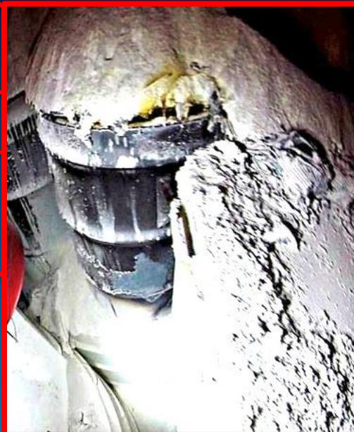
a matrix of organic kitty litter (fuel) with sodium nitrate (oxidizer) [reaction temperature: 300 °C]
