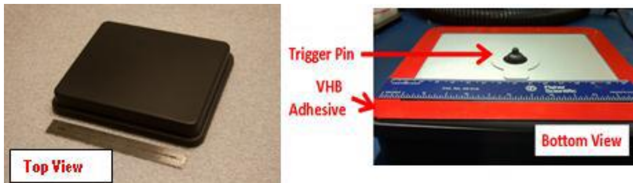
Figure 2: Bottom view of the secure passive tag shows the trigger pin to activate the miniature guillotine for self-destruction mode.
