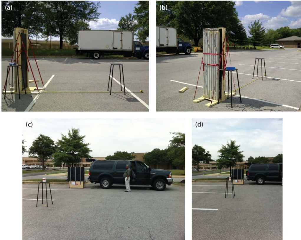
Figure 4. (a) The shielding side of the 6' \times 2'' ^3\text{He} tube array, (b) the detector side of the 6' \times 2'' tube array, (c and d) two mobile neutron pods facing the source. The detectors, shielding elements, and the source were always centered about 1 meter above ground.
