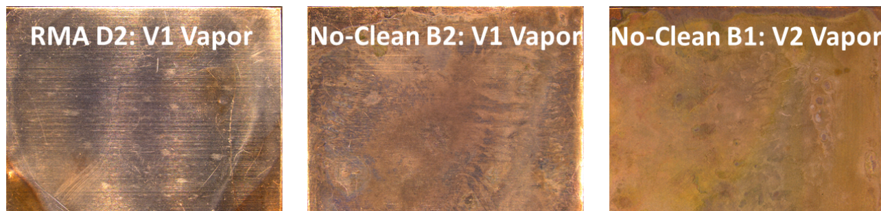
Figure 6. Best of High Temperature, no-clean flux B1 & B2 or RMA Flux D2.
