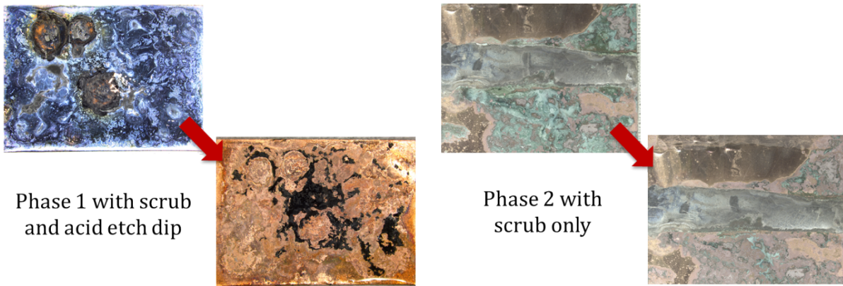
Figure 1. Post aging coupons cleaned to observe degree of etching.
