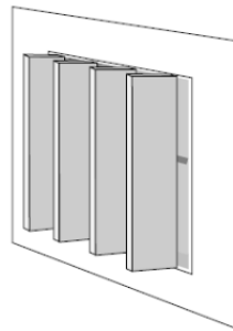
Figure 20: Vertical louvers or fins for east, and especially west, facades
