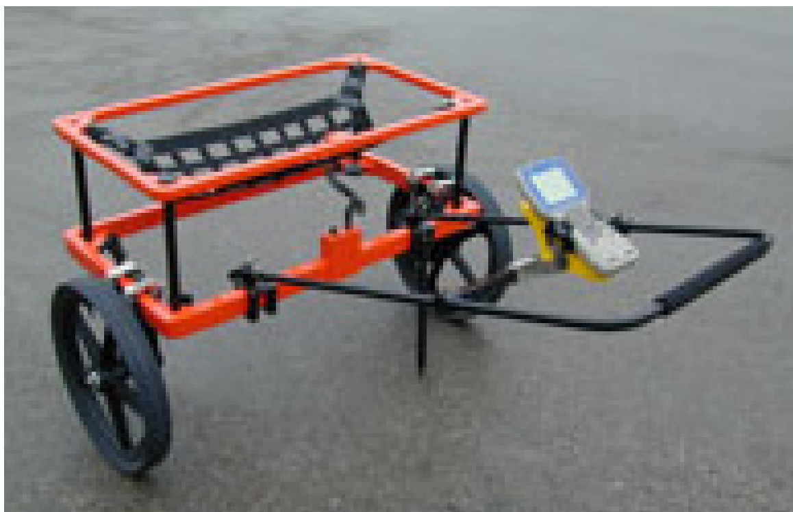
Figure G.2-2 Photo of the EM61-MK2A with Wheels Supporting Coils (Geonics, 2012)
