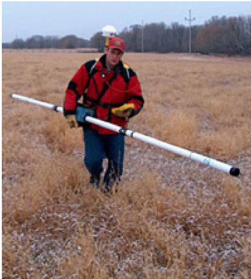
Figure G.2-1 Photo of the EM31-MK2 in Use Source: Geonics, 2012
