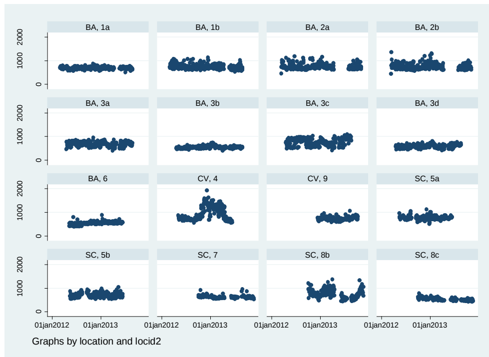
Figure 2. Daily CO 2 maximum indoor values over time (y-axis, in ppm, per study space grouped by climate zone)
