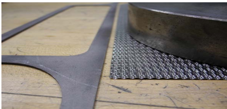
Figure 2-26 Anode Flow Field Fin with Fuel By-Pass Gap
