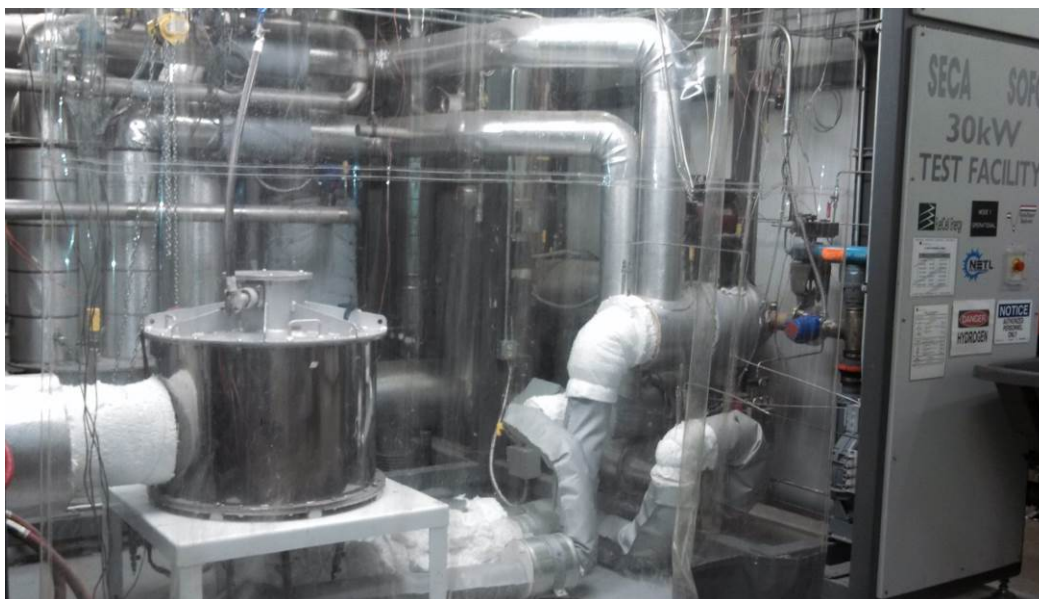
Figure 3-32 Modified 30 kW Facility with a 16-cell Stack Module Installed for Testing
