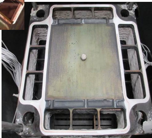
Figure 3-15 Comparison of Two Conductive Gasket Configurations Evaluated
