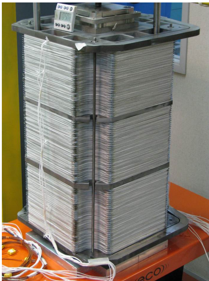
Figure 2-5 92-cell SOFC Stack Building Block (550 cm 2 cell active area)
