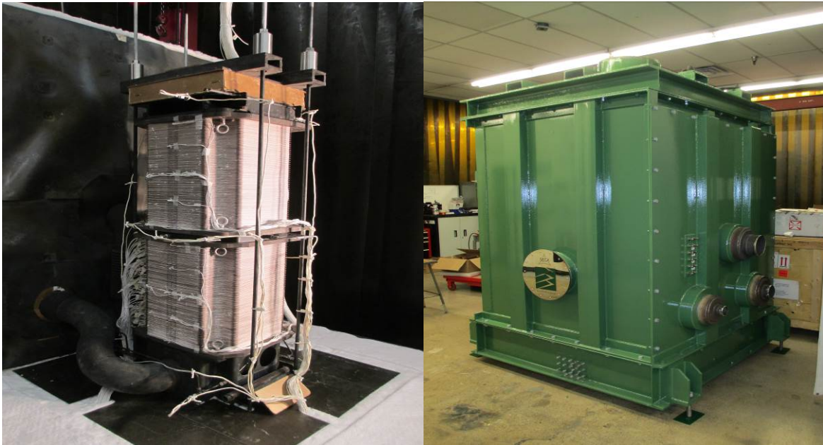
Figure 3-17 SO-30-5 Stack Tower (Two 96-cell Blocks, 550 cm 2 Active Area Cells) and Module Enclosure Assembly
