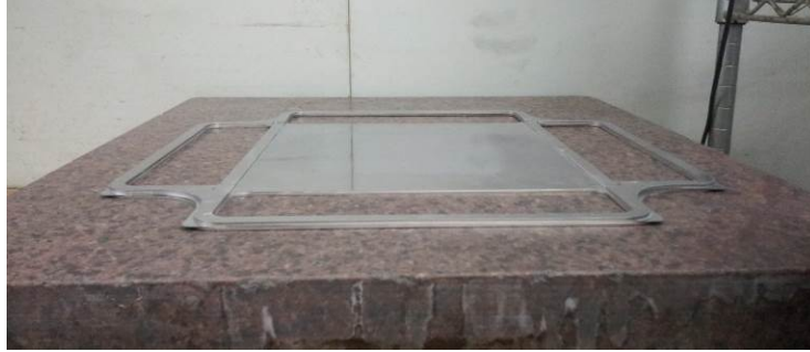
Figure 2-33 Brazed IC after Modifying Braze Furnace Temperature-Time Profile
