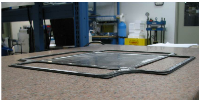
Figure 2-32 Brazed IC after Annealing
