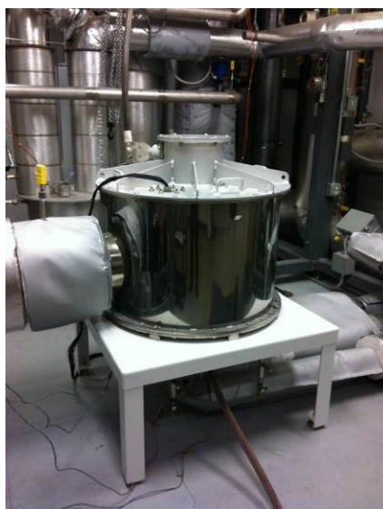
Figure 3-13 3-5 kW Module (Containing 16-cell SOFC Stack) Integrated into the 30 kW Test Facility
