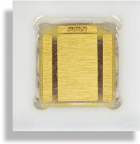
Figure 2: Back side view of high-power white LED package.
